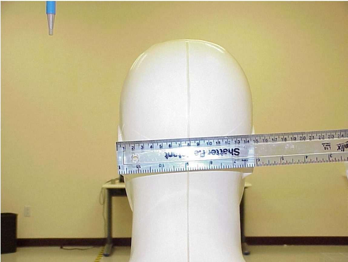
Photo 8. Photo to demonstrate 15 cm Z-axis head phantom
