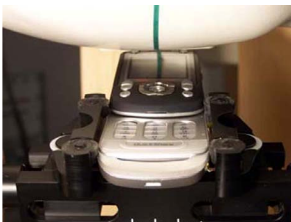
Device position against the head: Tilt (cheek+15deg) phone position (phone in open state)
