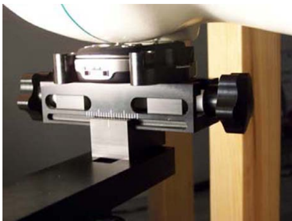
Device position against the head: Cheek (touch) phone position (phone in close state)
