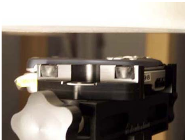
Device position against the body: Phone in close state
