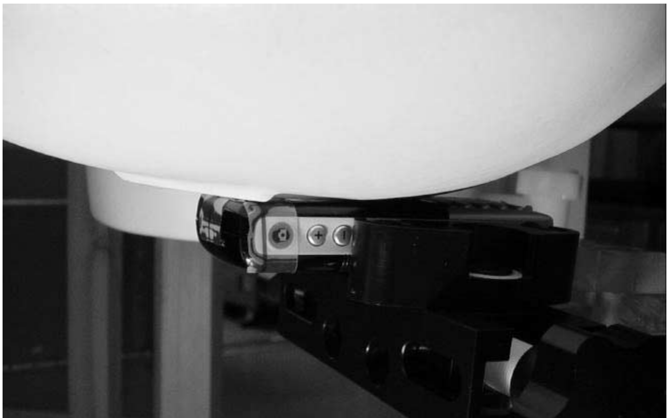
Position of device against head phantom using the “cheek” position
