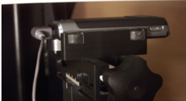
Device position against the body: 15mm distance from Phantom.
