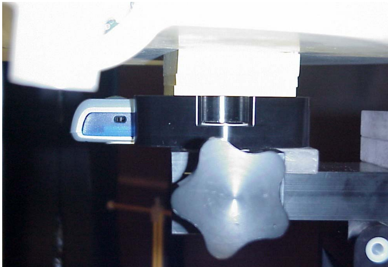
Position of device against flat phantom using a 20 mm spacer with hands free accessory RLF 501 25/04 (HPE-14).
