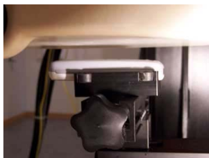
Device position against the body: Phone with 15mm distance against flat section of the phantom.
