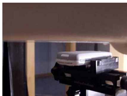
Device position against the body: Phone with 15mm distance against flat section of the phantom.
