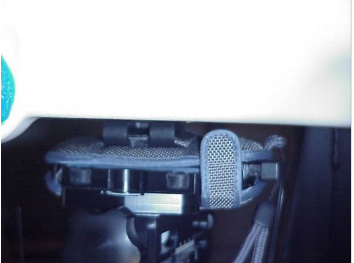
Position of device against flat phantom using carry accessory ICT14 with hands free accessory (HPB-20).
