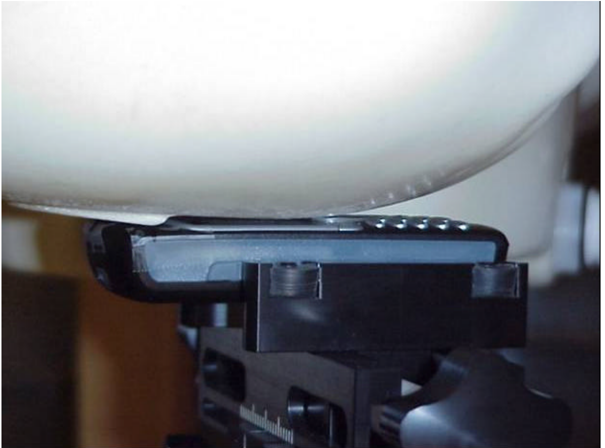
Position of device against head phantom
