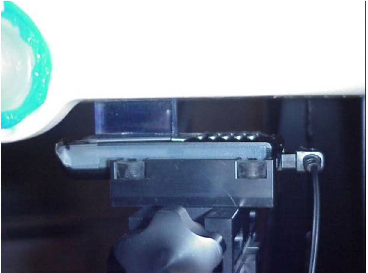
Position of device against flat phantom using a 15mm spacer with hands free accessory (HPB-20).
