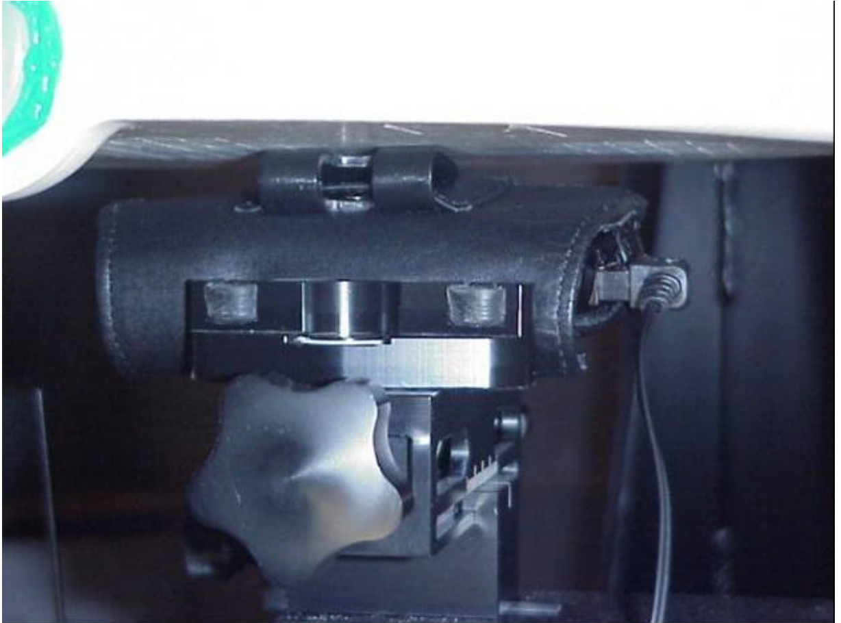
Position of device against flat phantom using carry accessory ICE25 with hands free accessory (HPB-20).
