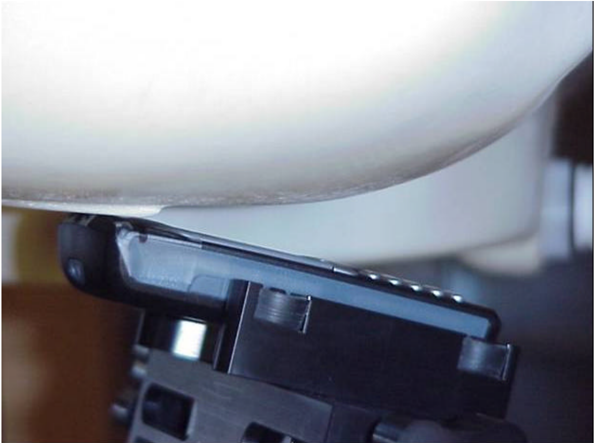
Position of device against head phantom in the tilted position
