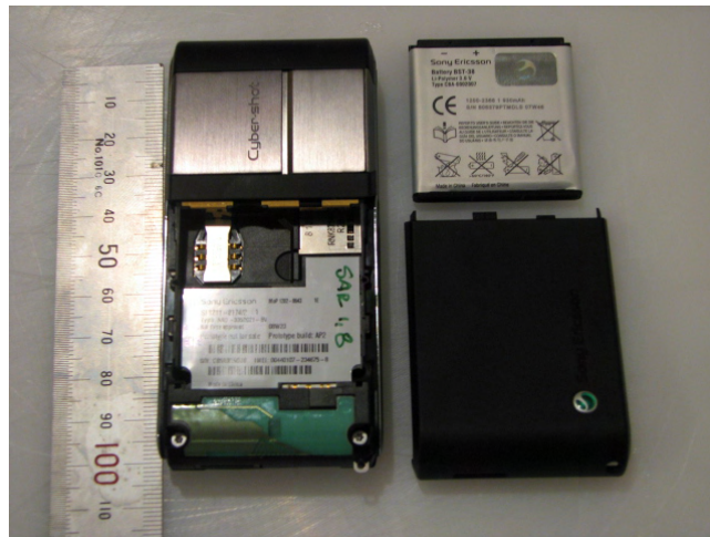
Battery and cover removed
