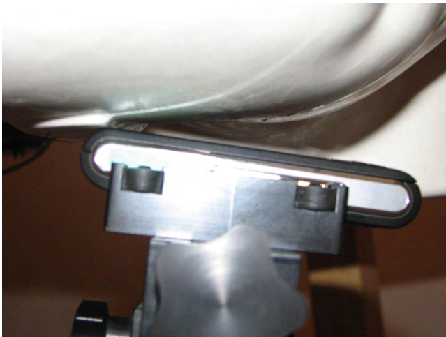
DUT position towards the head: Tilt (touch + 15°) position
