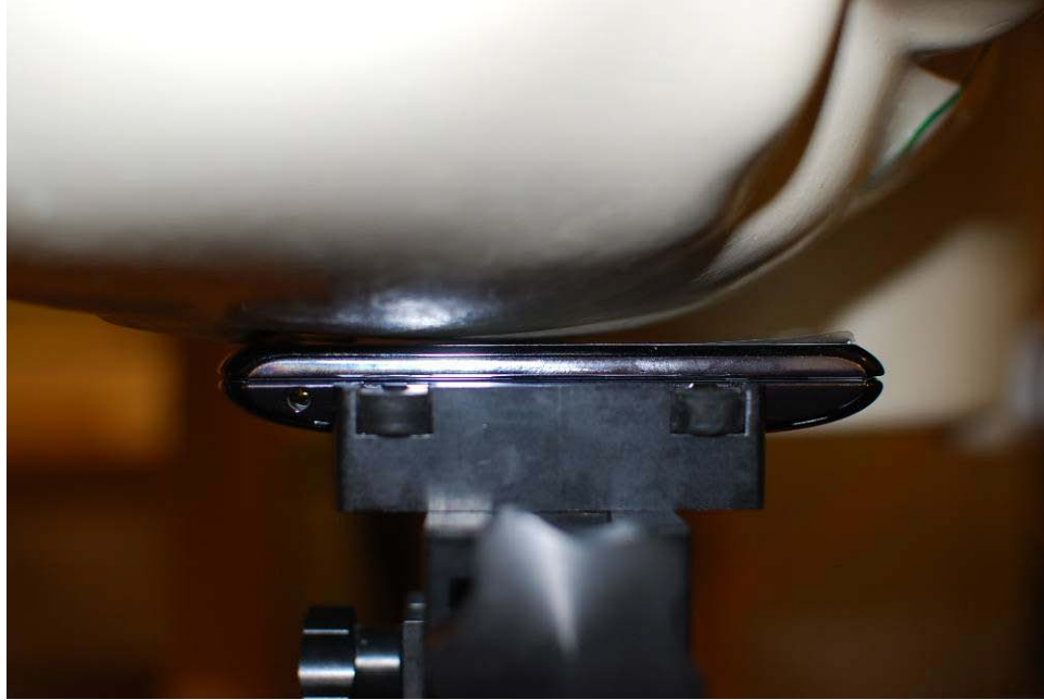
Figure 21-3 SAR Test Setup Photo – Right Touch
