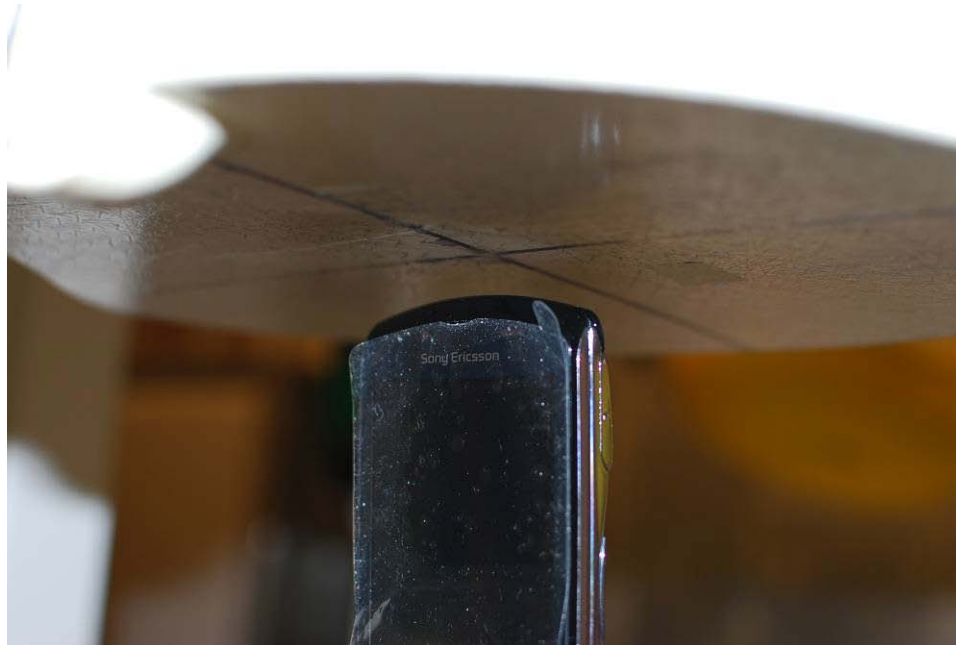
Figure 21-7 SAR Test Setup Photo – Top at 1.0 cm
