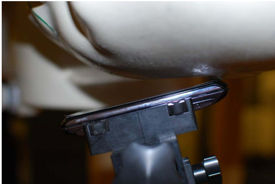
Figure 21-2 SAR Test Setup Photo – Left Tilt
