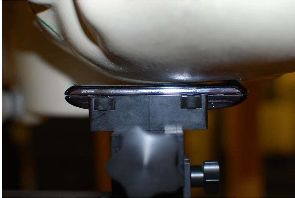
Figure 21-1 SAR Test Setup Photo – Left Touch
