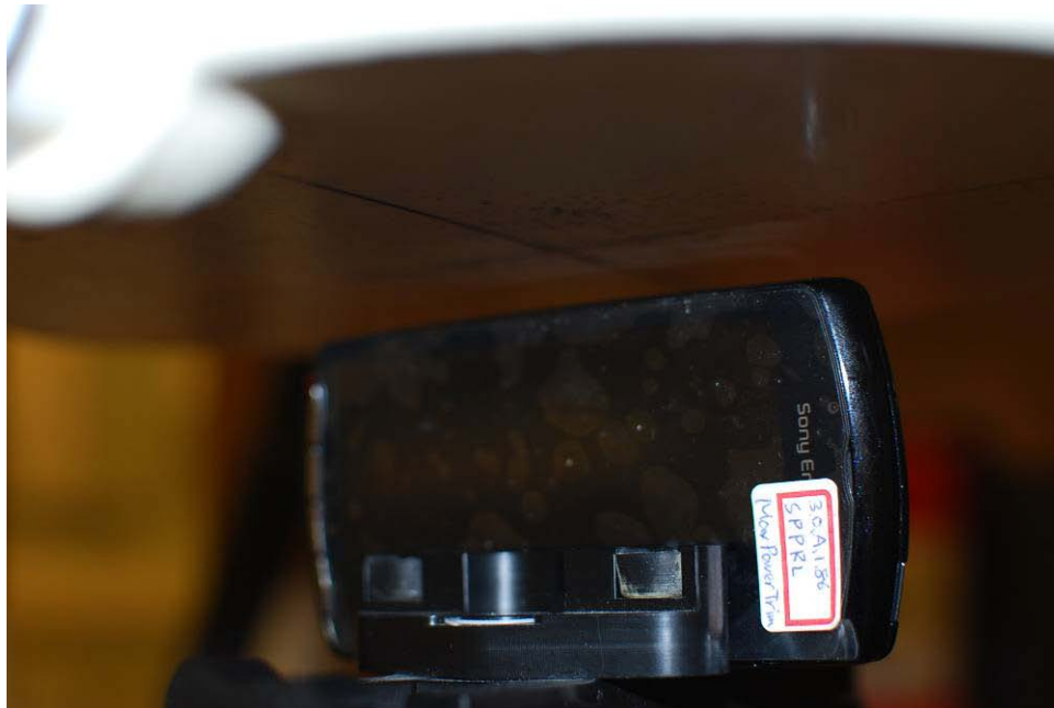
Figure 21-10 SAR Test Setup Photo – Left at 1.0 cm
