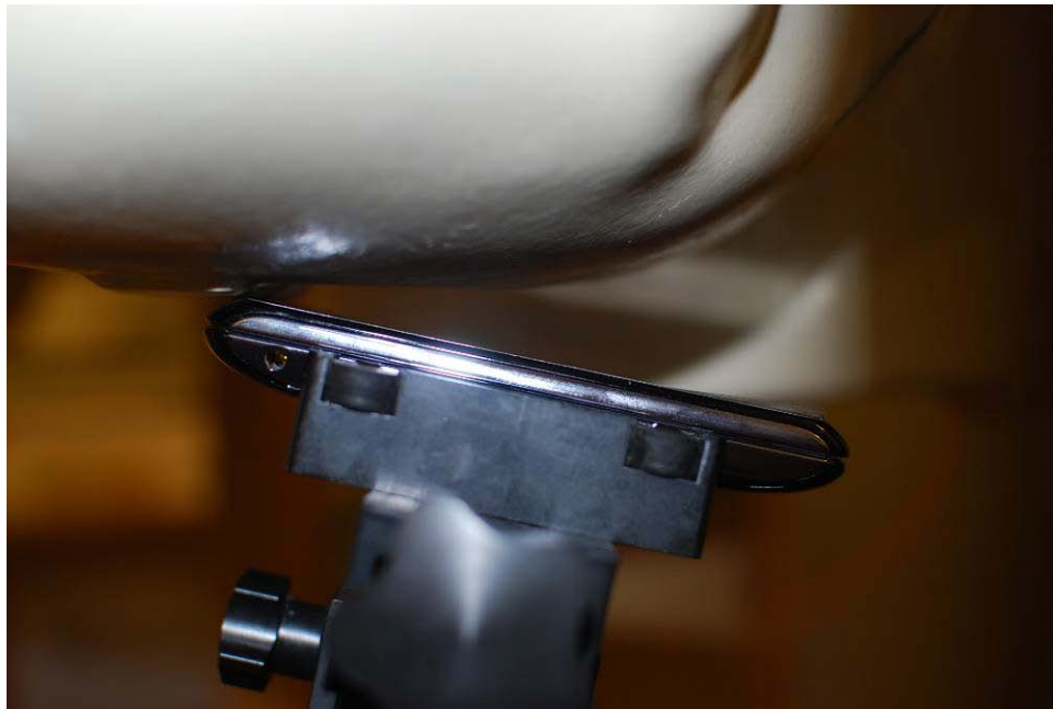
Figure 21-4 SAR Test Setup Photo – Right Tilt
