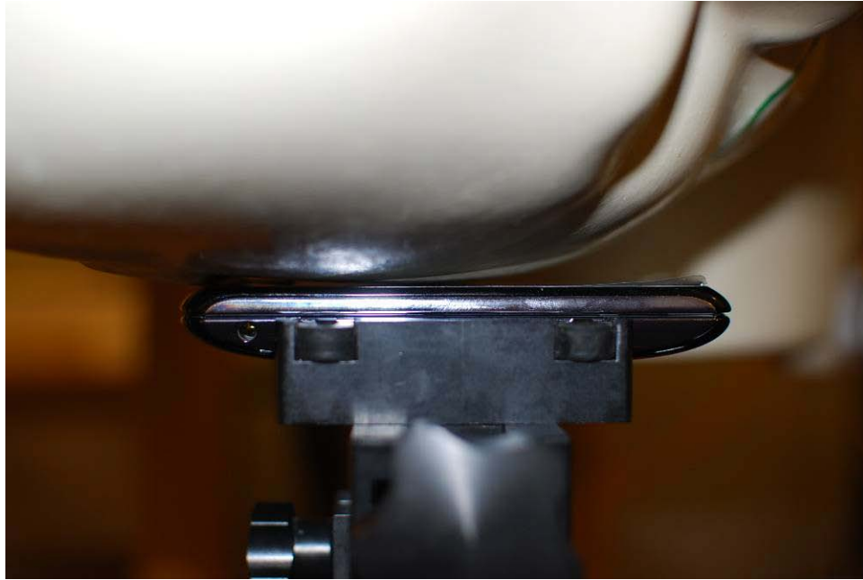
Figure 21-3 SAR Test Setup Photo – Right Touch
