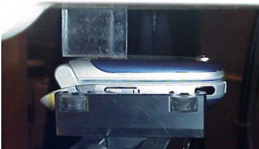
Position with front of device against flat phantom closed using a 25MM SPACER for PTT.
