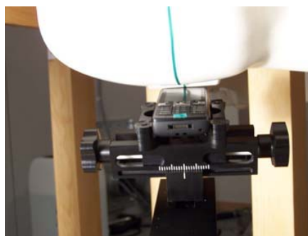
Device position against the head: Tilt (cheek+15deg) phone position
