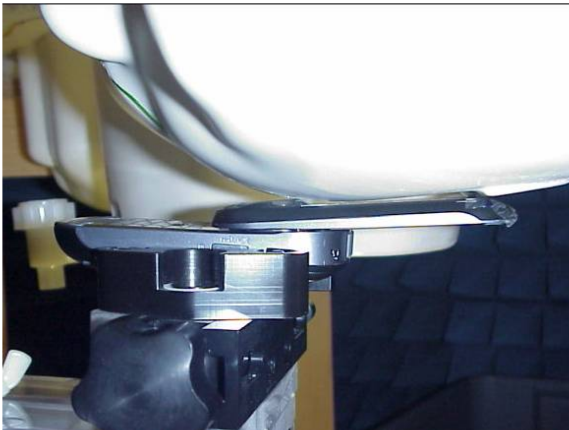
Position of device against head phantom in open position
