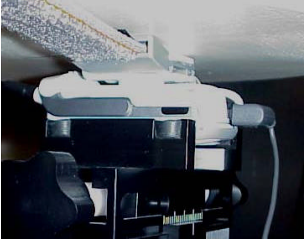
Position of device against body phantom with IAC60 in back position.
