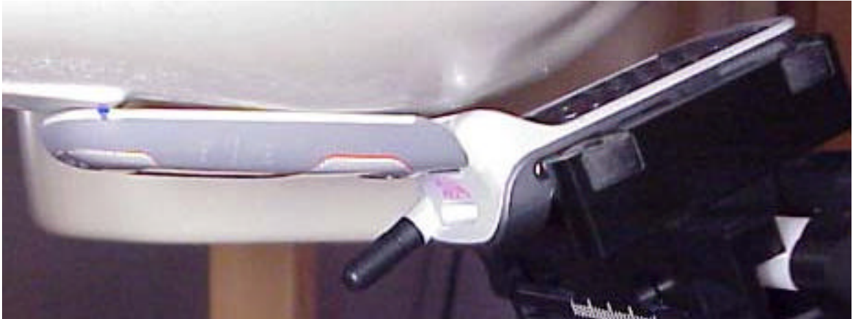
Position of device against head phantom using the “cheek” position
