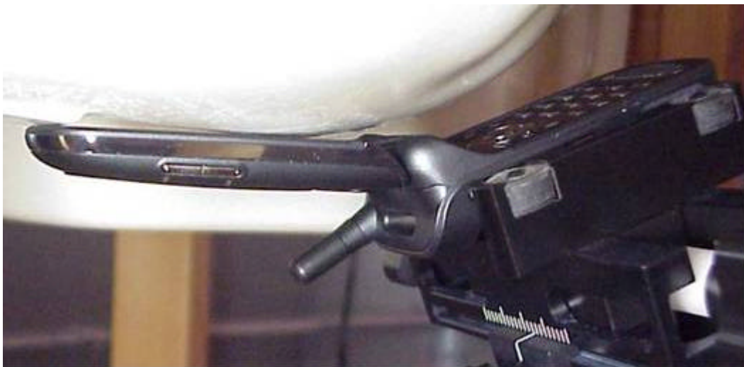
Position of device against head phantom using the “cheek” position
