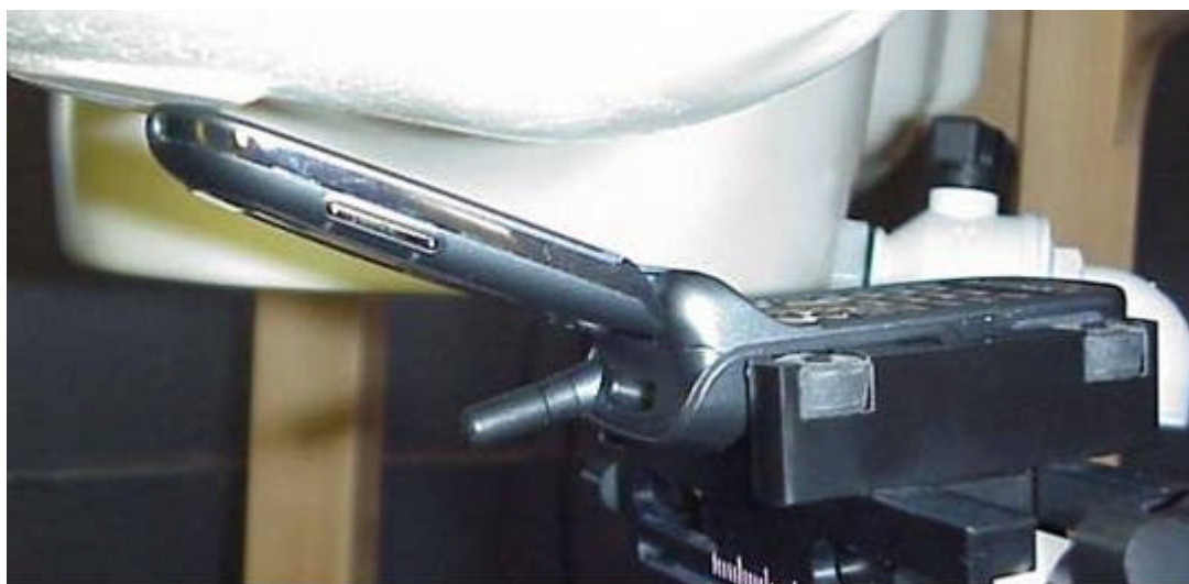
Position of device against head phantom using the “tilt” position
