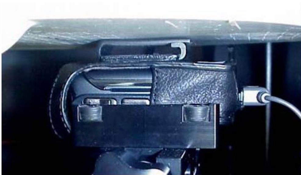
Position of device against body phantom with ICE26 in front position.
