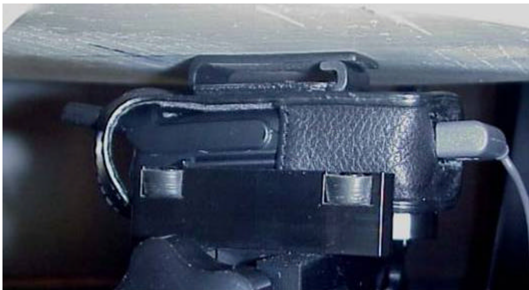
Position of device against body phantom with ICE26 in back position.
