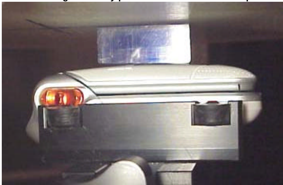
Position of device against body phantom with ICE26 in back position.
