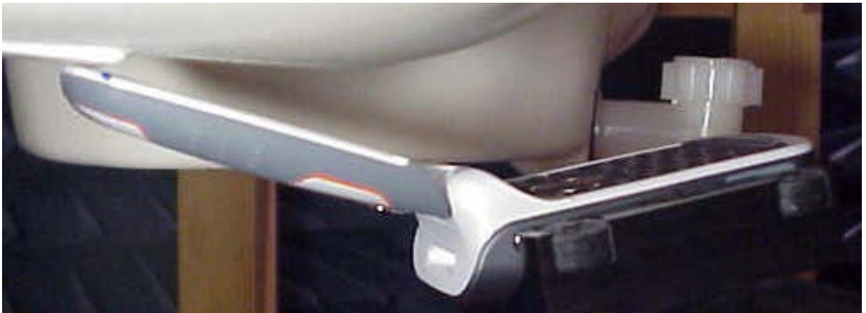
Position of device against head phantom using the “tilt” position
