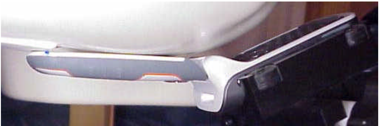
Position of device against head phantom using the “cheek” position
