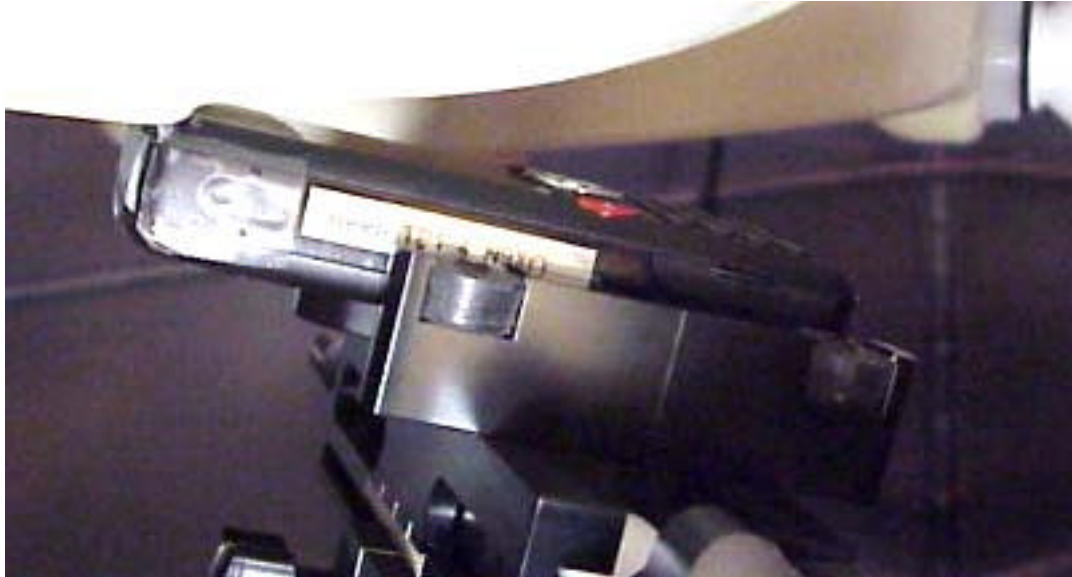
Position of device against head phantom using the “tilt” position
