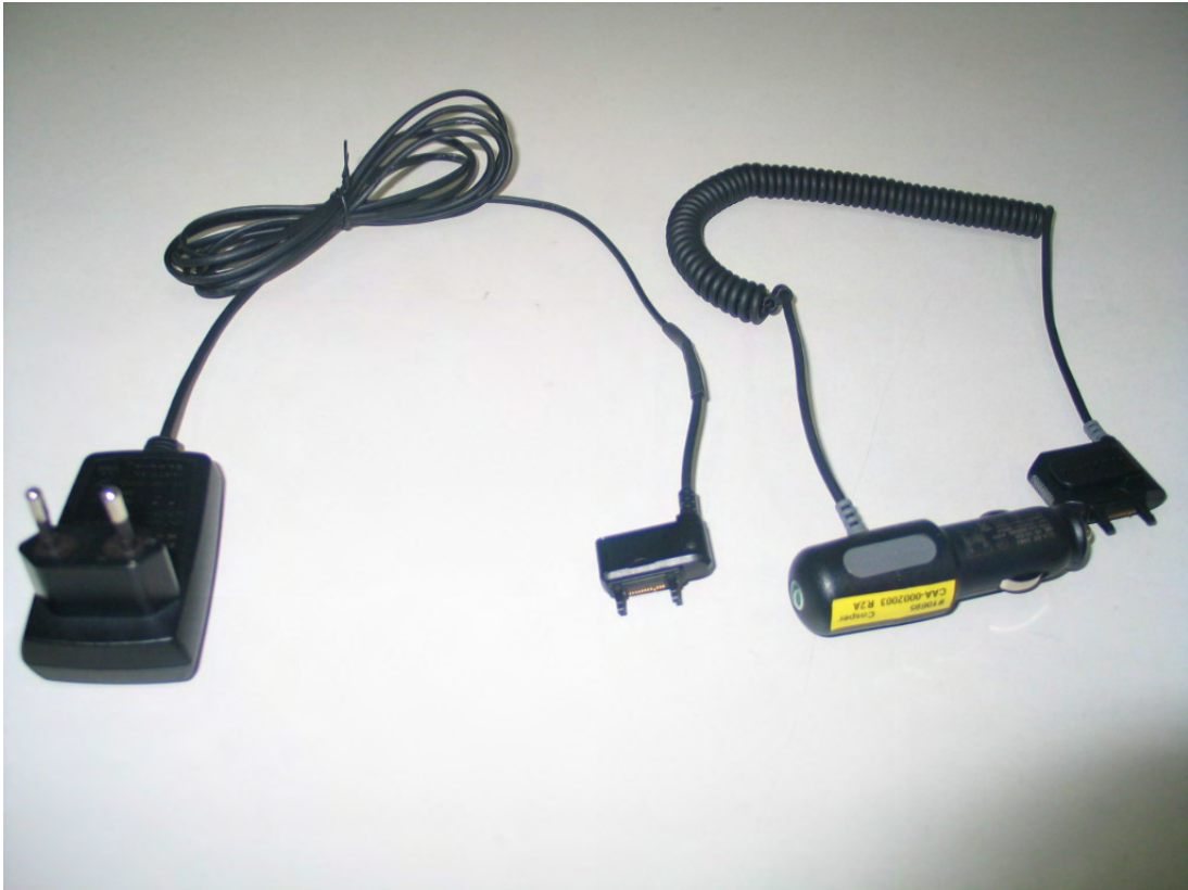
Photo 7: Ancillary Equipment (AC travel charger 13200AC02, DC vehicular charger 13200DC02)
