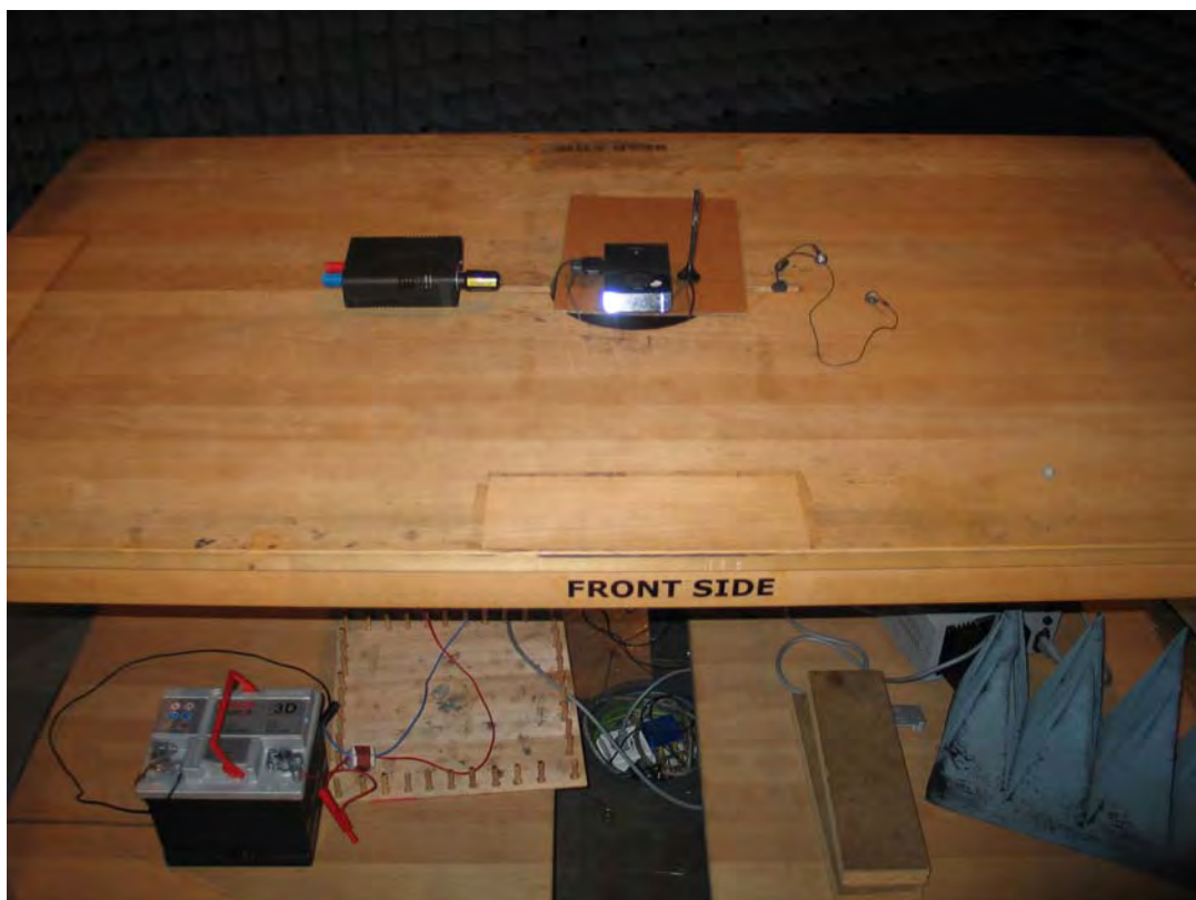
Photo 2: Test setup for radiated measurements below 1GHz (setup AD_03)
