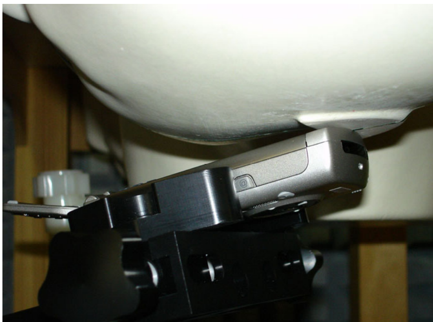
(b) Device on head phantom in the tilt position with the flip open.
