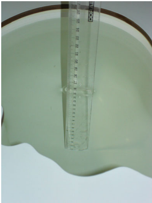
Measured level of 2450 MHz head tissue simulating liquid in phantom
