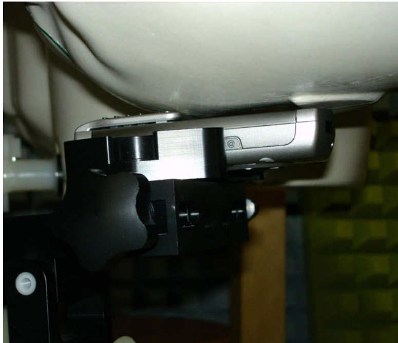
(a) Device on head phantom in the cheek position with the flip closed.
