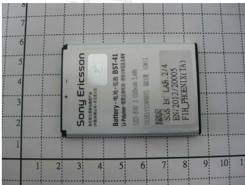
Fig.18 Front view of battery (Model No.: BST-41, Supplier: SONY, Type No.: CBA-0002012)
