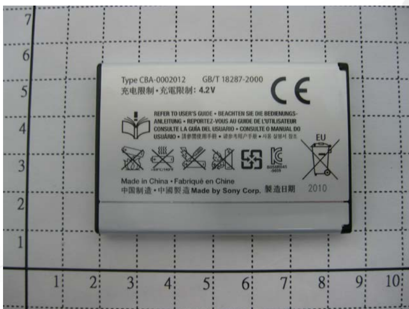
Fig.19 Back view of battery (Model No.: BST-41, Supplier: SONY, Type No.: CBA-0002012)
