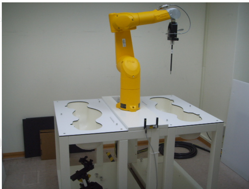
Fig.1 Photograph of the SAR Measurement System
