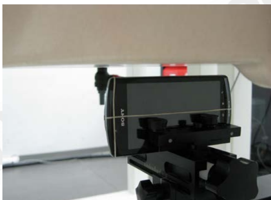
Fig.13 EUT Right to flat phantom
