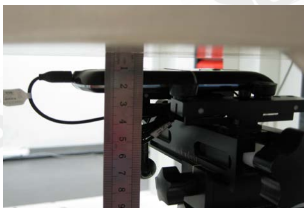
Fig.11 EUT Back side with Headset to flat phantom
