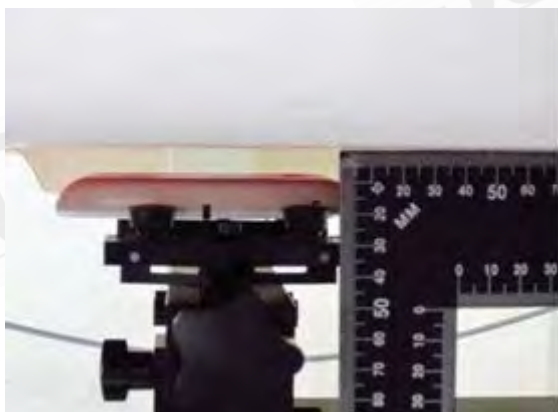
Fig.10 EUT back to flat phantom
