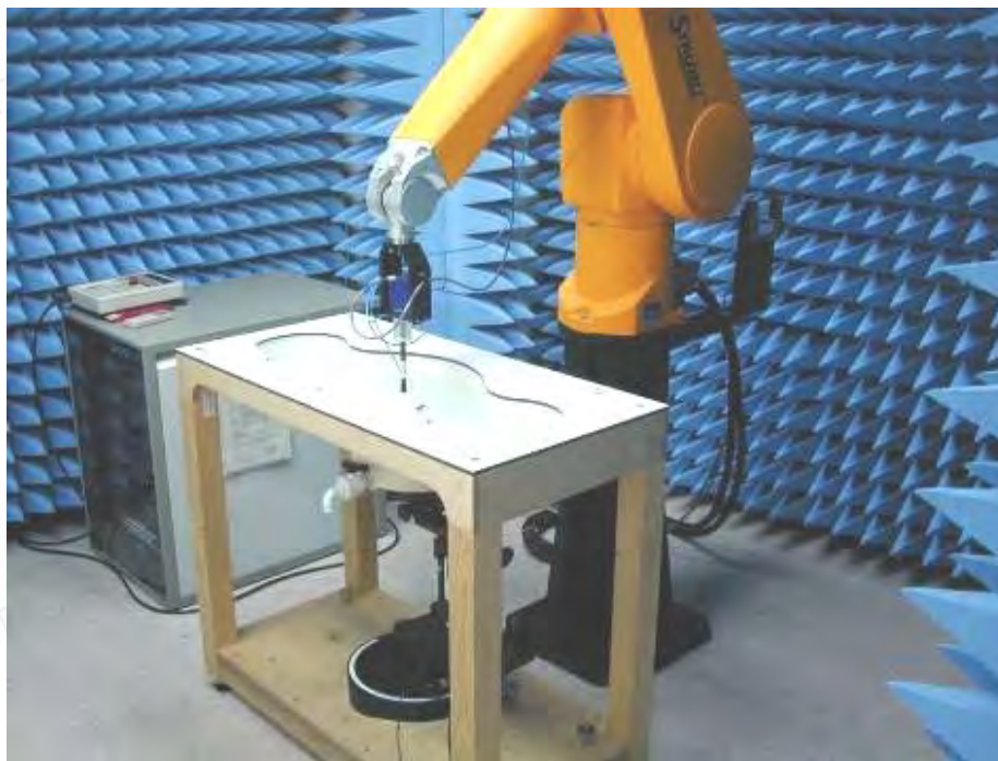
Fig.1 Photograph of the SAR measurement System
