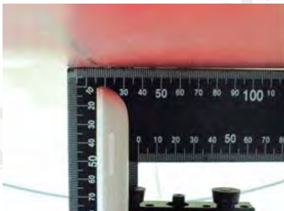
Fig.12 EUT Top to flat phantom
