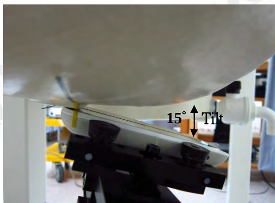
Fig.4 Right Head Section / Ear-Tilt Position(15°)
