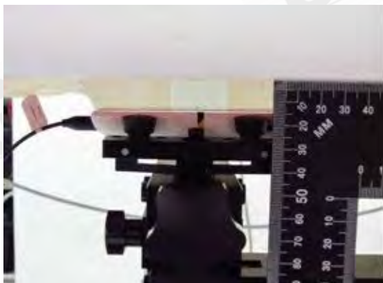
Fig.7 EUT Front side with Headset to flat phantom
