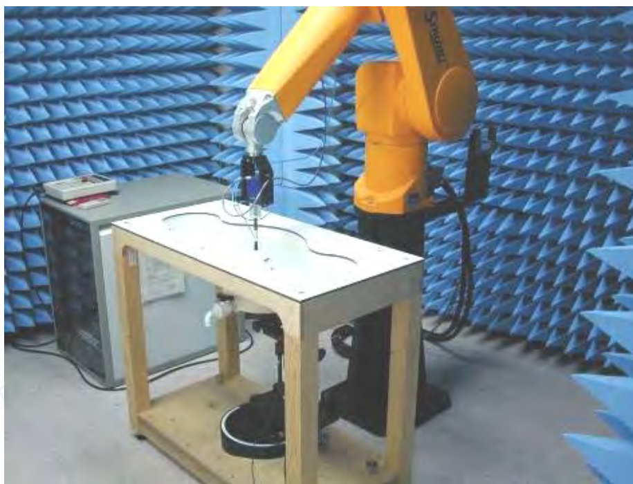
Fig.1 Photograph of the SAR measurement system
