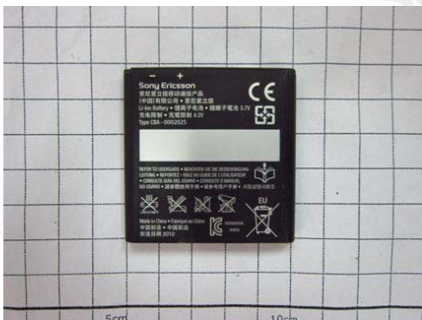
Fig.19 Back view of Battery (Model No.: BA700, Supplier: Sony, Manufacture: LG, Type No.: CBA-0002025)
