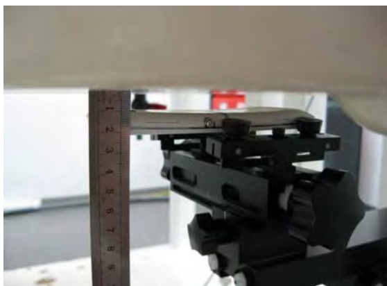
Fig.10 EUT back to flat phantom
