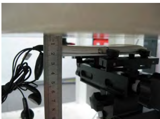
Fig.11 EUT back side with headset (MH410C) to flat phantom
