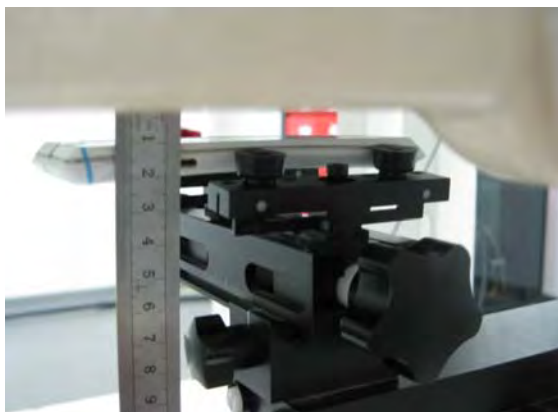
Fig.9 EUT front to flat phantom
