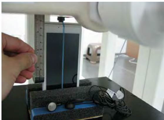
Fig.12 EUT bottom with headset (MH410C) to flat phantom
