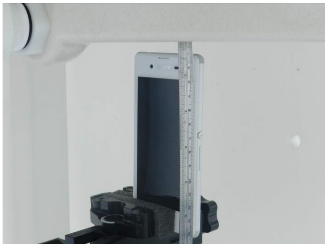
Top Side, Test Separation 1.0 cm
