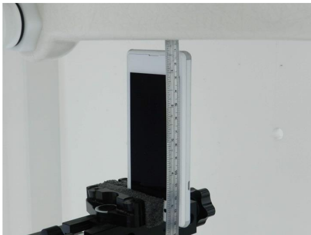
Bottom Side, Test Separation 1.0 cm
