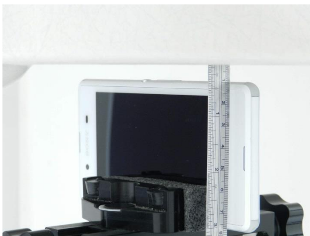
Right Side, Test Separation 1.0 cm
