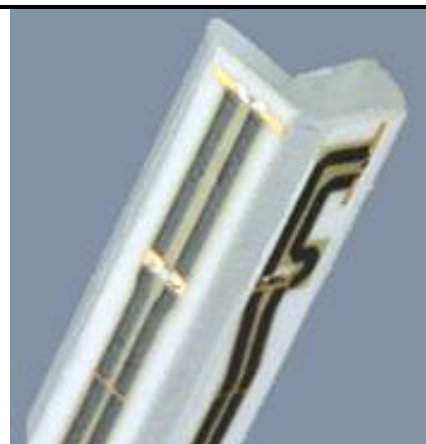
Fig 5.2 Photo of E-field Probe
