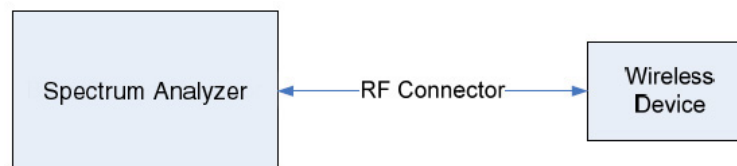
Figure 6-1. Test Instrument & Measurement Setup
