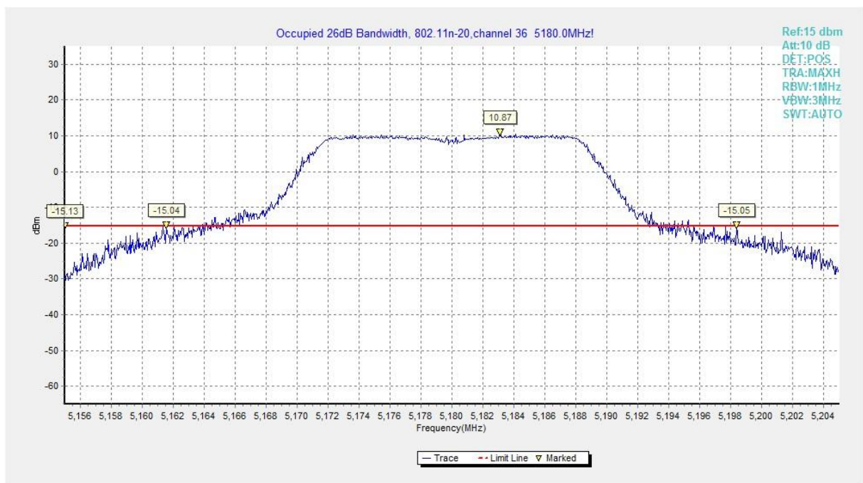
Fig. 10 Occupied 26dB Bandwidth (802.11n-HT20, 5180MHz)
