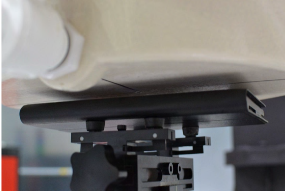
SAR Test Setup Photo 9 – Back Side at 1.0 cm with L-Battery Cover
