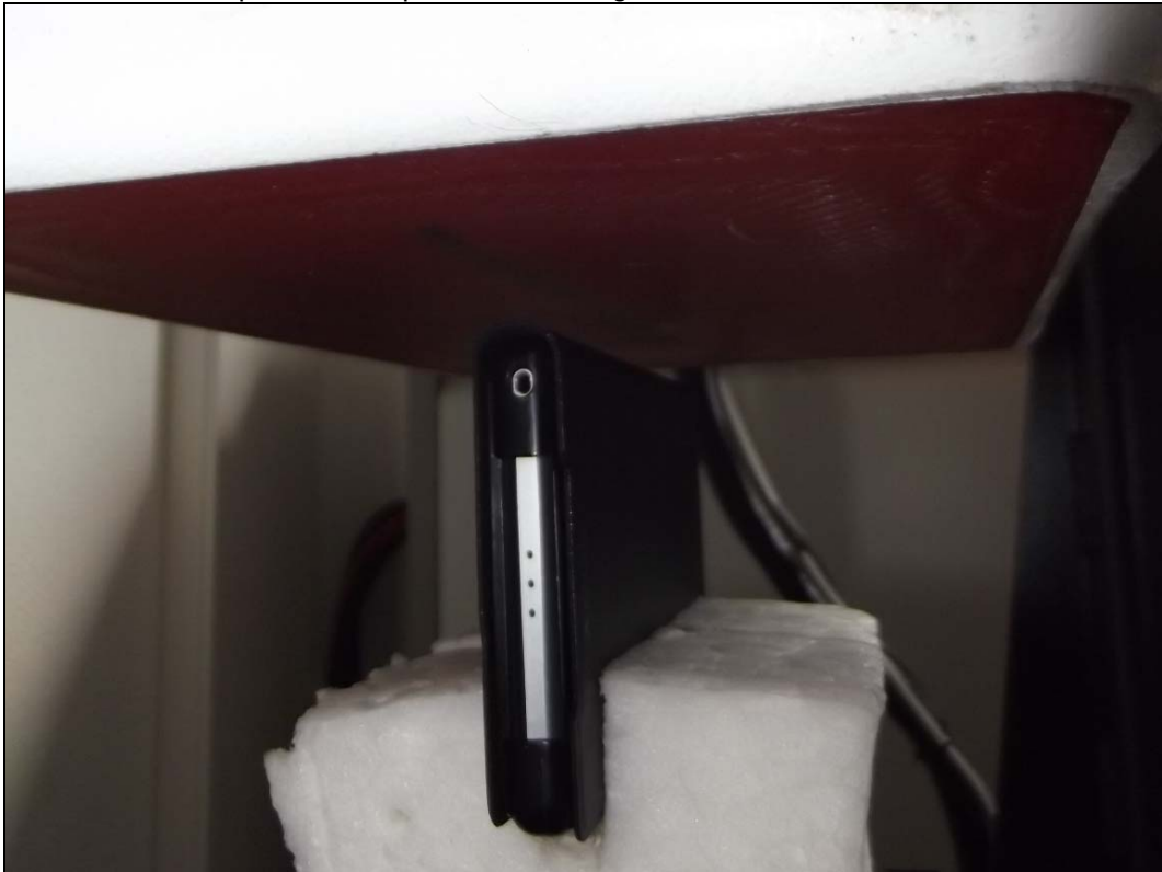
Photo 26: Test position hotspot mode right edge side 10mm distance with WPC cover
