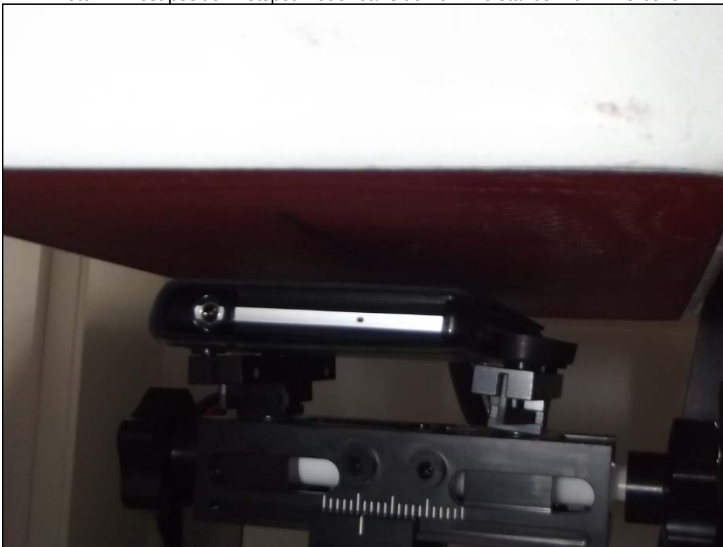
Photo 24: Test position hotspot mode rear side 10mm distance with WPC cover
