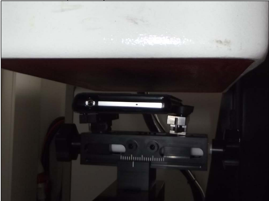
Photo 28: Test position body worn rear side 15mm distance with WPC cover
