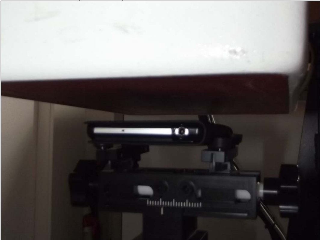
Photo 28: Test position body worn rear side 15mm distance with WPC cover
