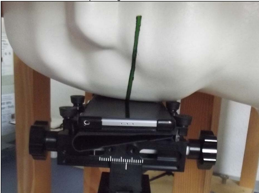
Photo 20: Test position right hand touched with WPC cover
