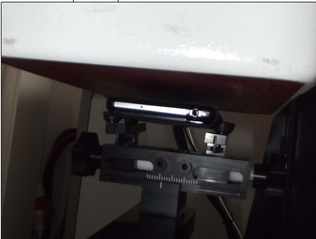
Photo 24: Test position hotspot mode rear side 10mm distance with WPC cover
