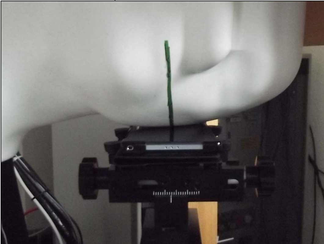
Photo 18: Test position left hand touched with WPC cover
