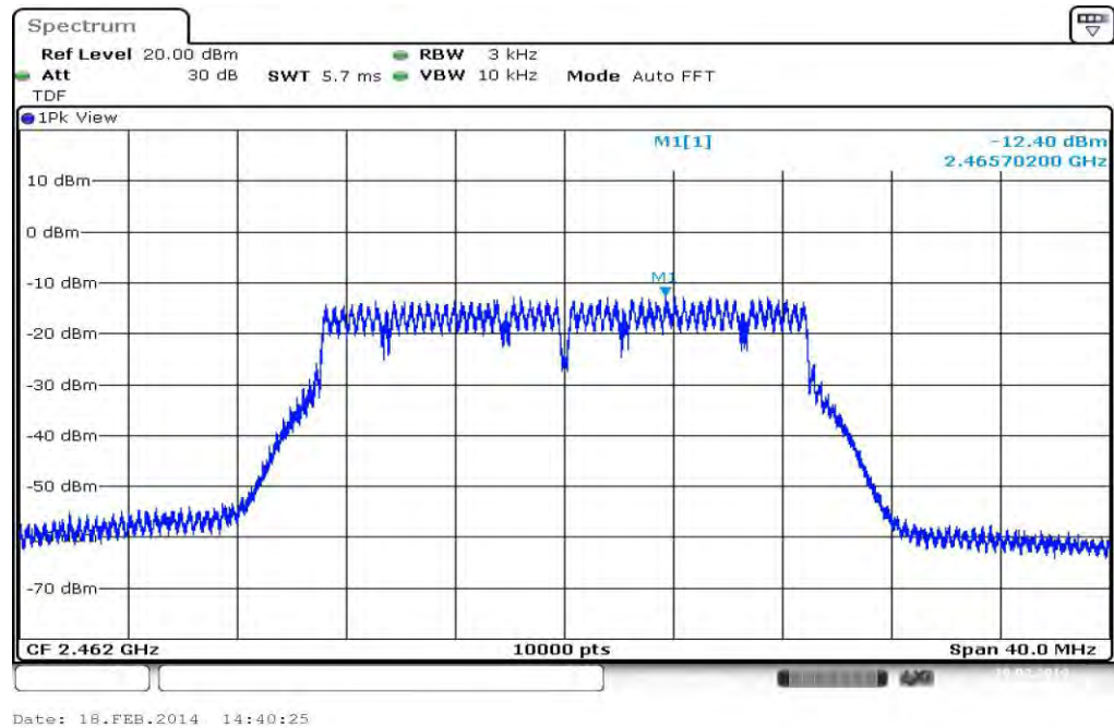
Plot 3: TX mode, highest channel
