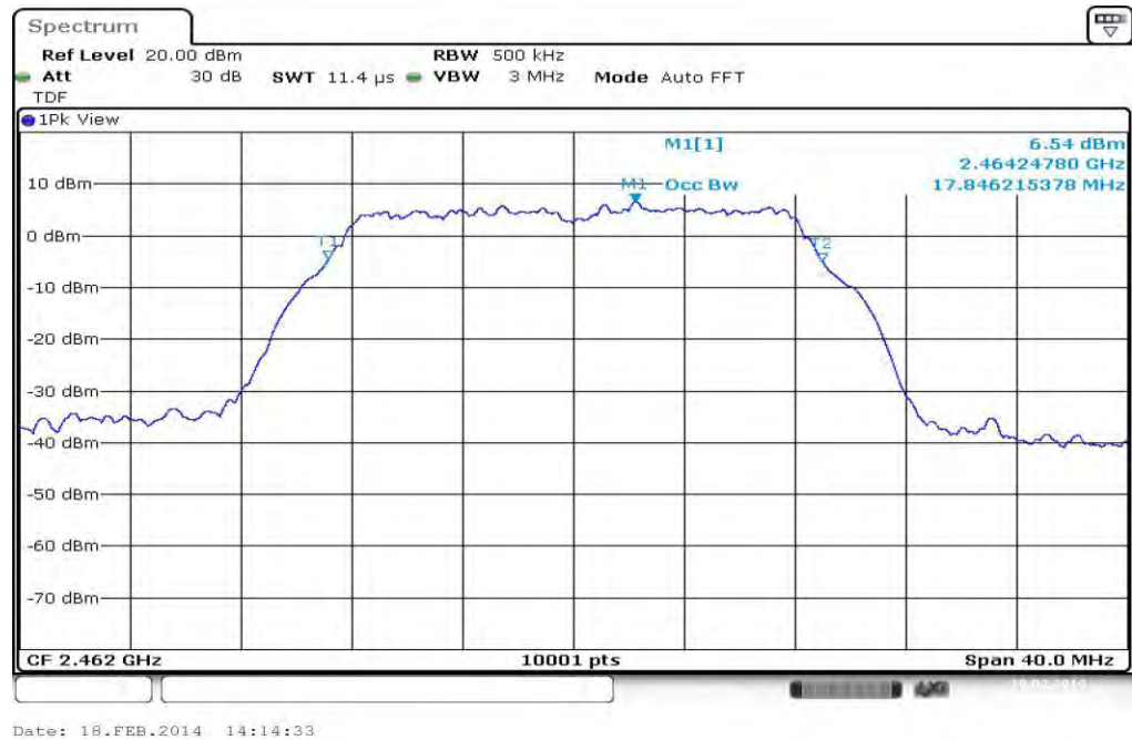
Plot 3: TX mode, highest channel
