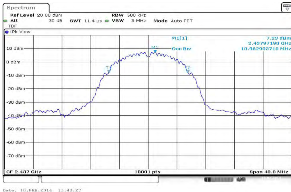
Plot 2: TX mode, middle channel
