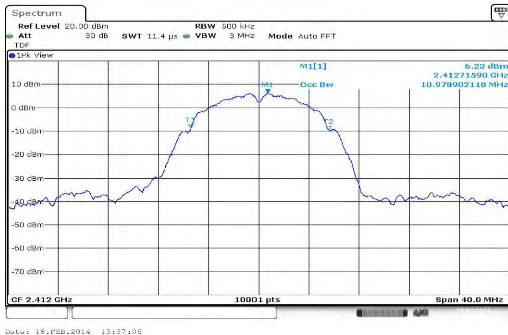
Plot 1: TX mode, lowest channel
