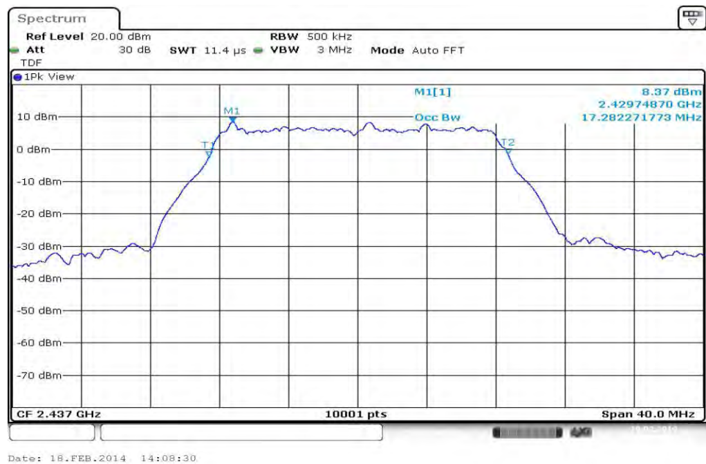
Plot 2: TX mode, middle channel
