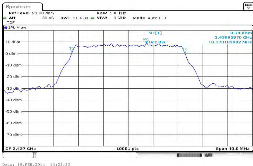
Plot 2: TX mode, middle channel
