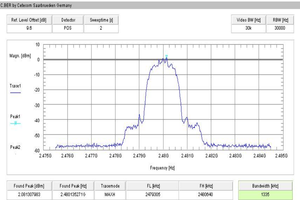
Plot 9: highest channel – 2480 MHz, 8 DPSK modulation
