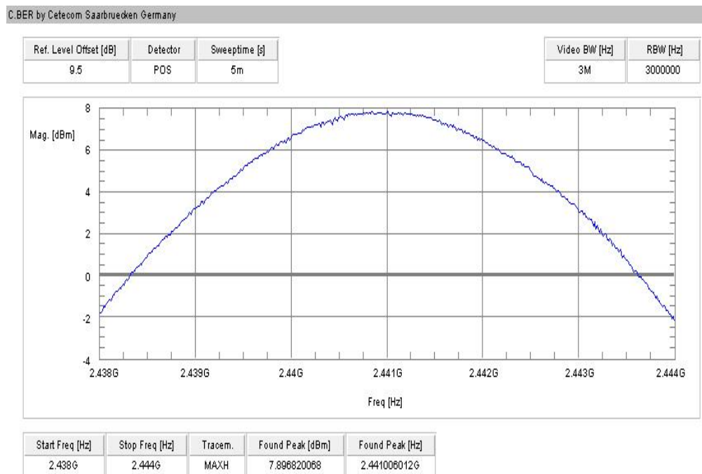
Plot 8: middle channel – 2441 MHz, 8 DPSK modulation
