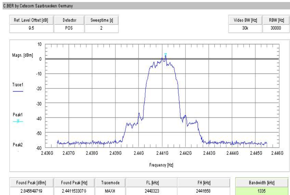
Plot 5: middle channel – 2441 MHz, Pi / DQPSK modulation
