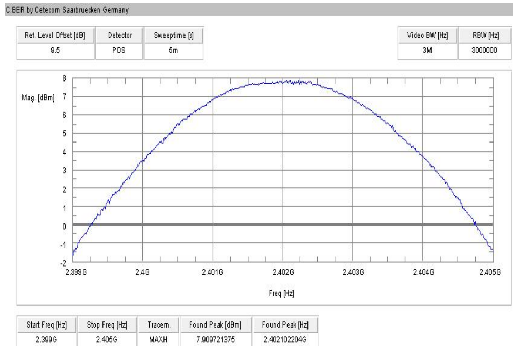
Plot 4: lowest channel – 2402 MHz, Pi / DQPSK modulation
