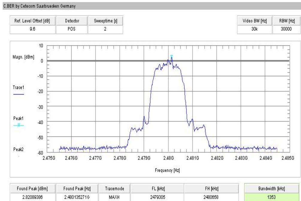
Plot 6: highest channel – 2480 MHz, Pi / DQPSK modulation
