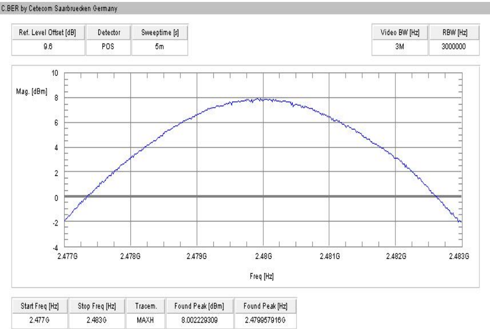
Plot 9: highest channel – 2480 MHz, 8 DPSK modulation
