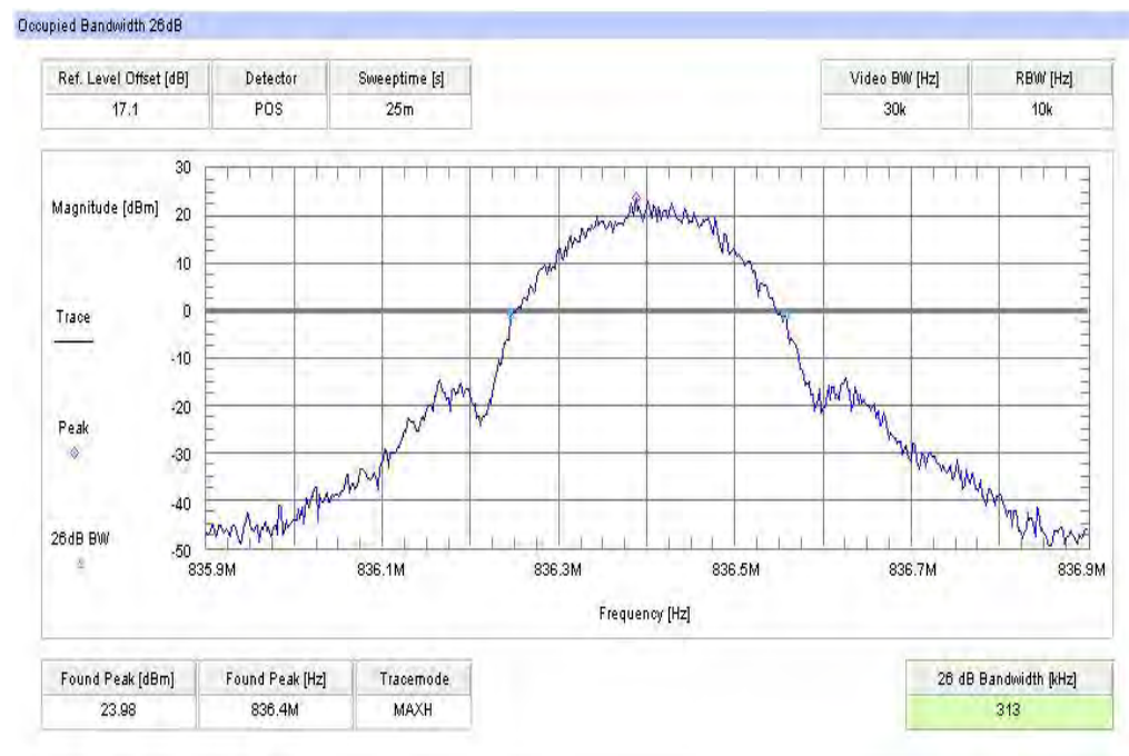
Plot 10: Channel 189 (-26 dBc BW) - 8-PSK
