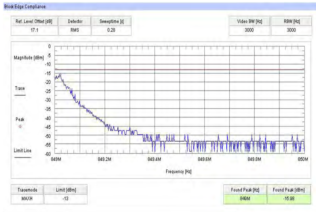
Plot 2: Channel 251 (GSM-mode)
