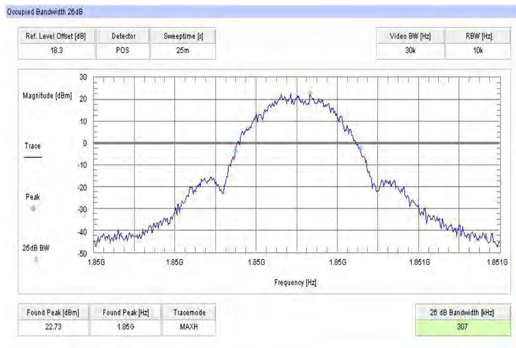
Plot 8: Channel 512 (-26 dBc BW) - EDGE
