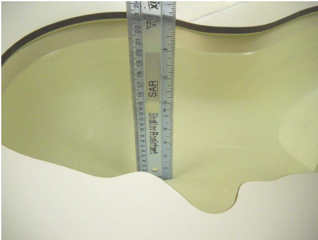
Photo 11: 15cm Liquid Depth in SAM head
