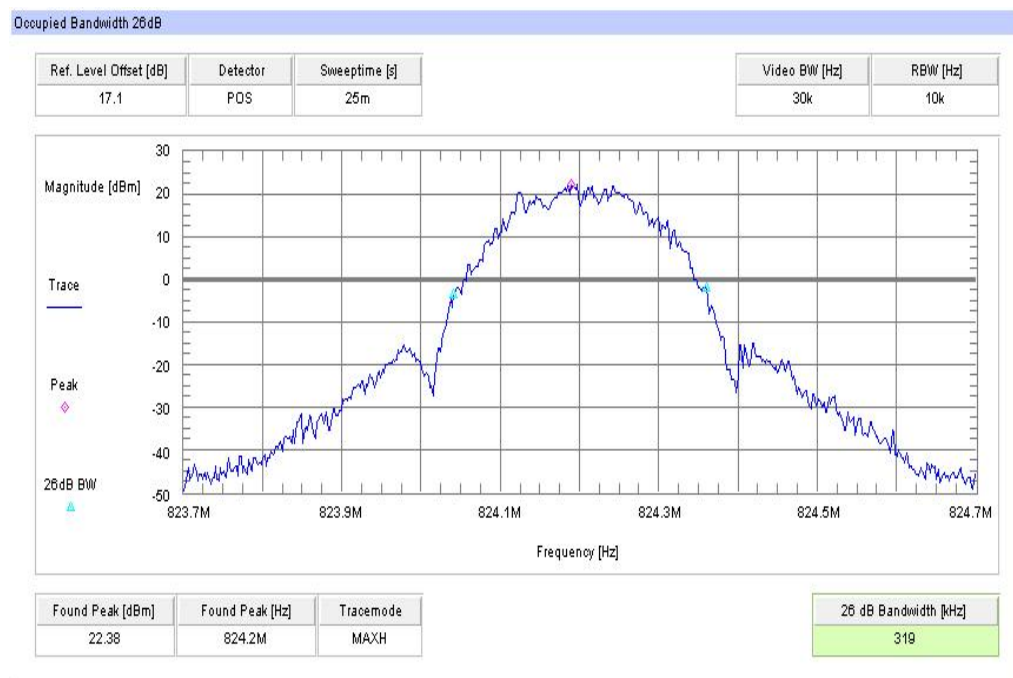
Plot 8: Channel 128 (-26 dBc BW) - 8-PSK
