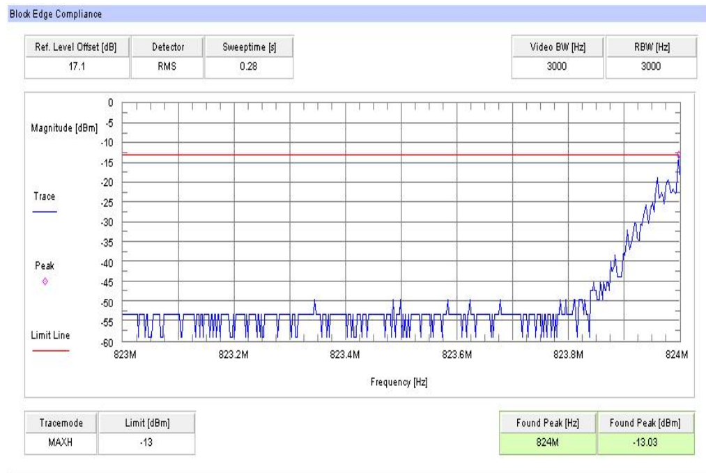
Plot 1: Channel 128 (GSM-mode)
