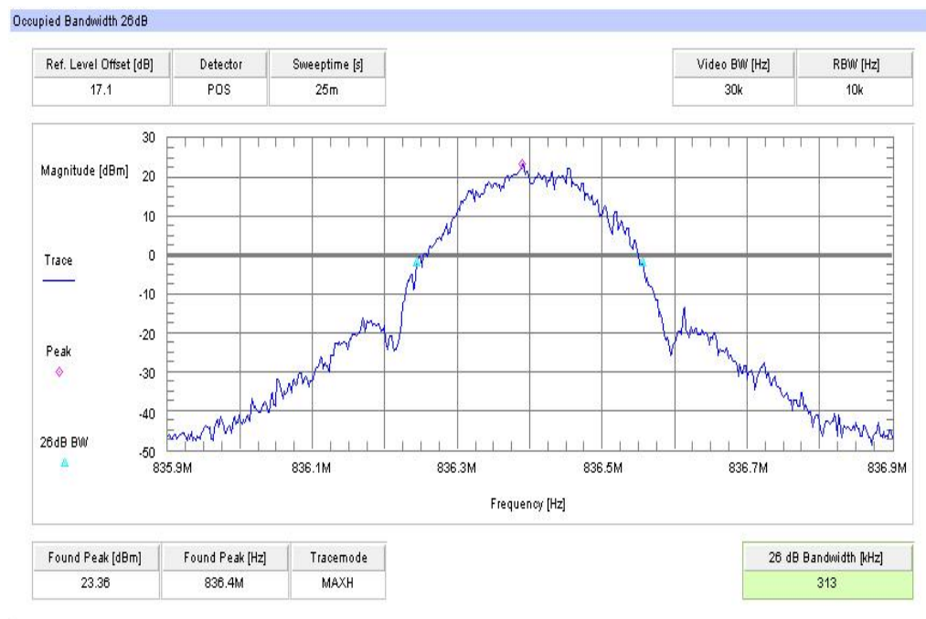
Plot 10: Channel 189 (-26 dBc BW) - 8-PSK
