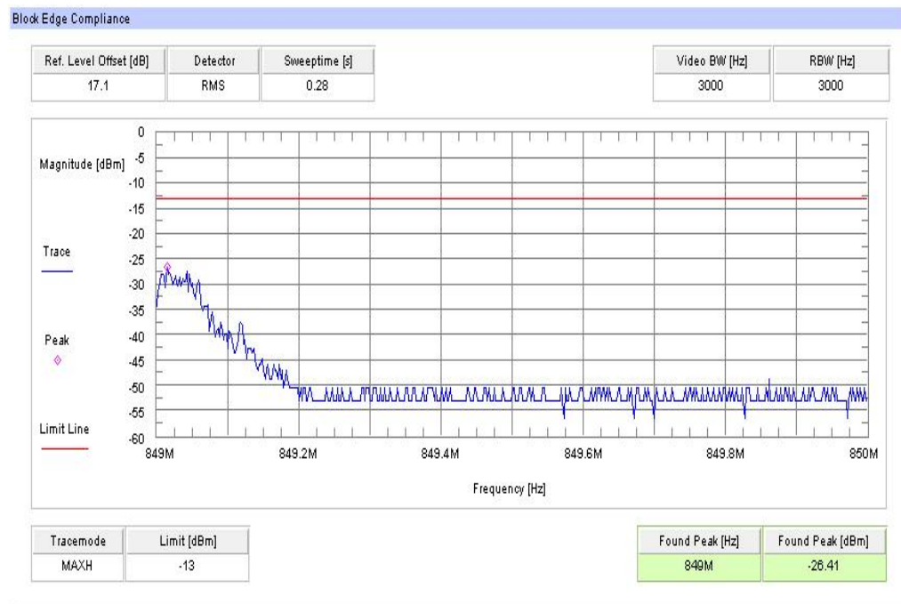
Plot 4: Channel 251 (EDGE-mode)
