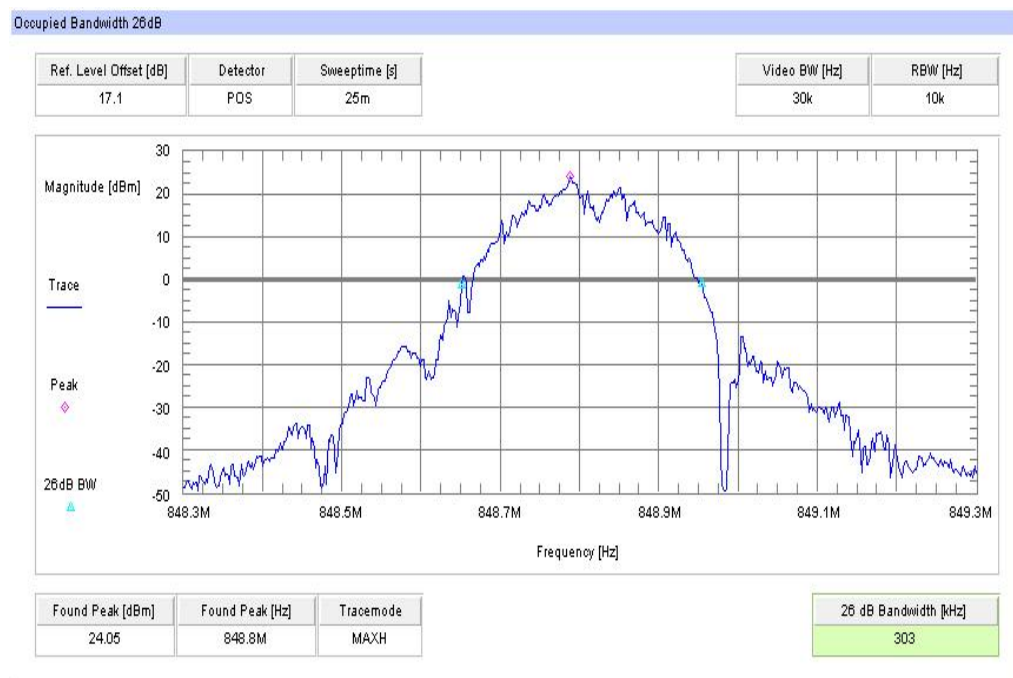
Plot 12: Channel 251 (-26 dBc BW) - 8-PSK
