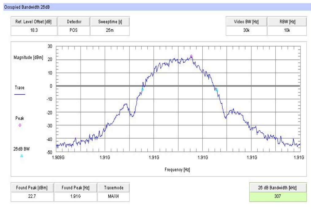
Plot 12: Channel 810 (-26 dBc BW) - EDGE
