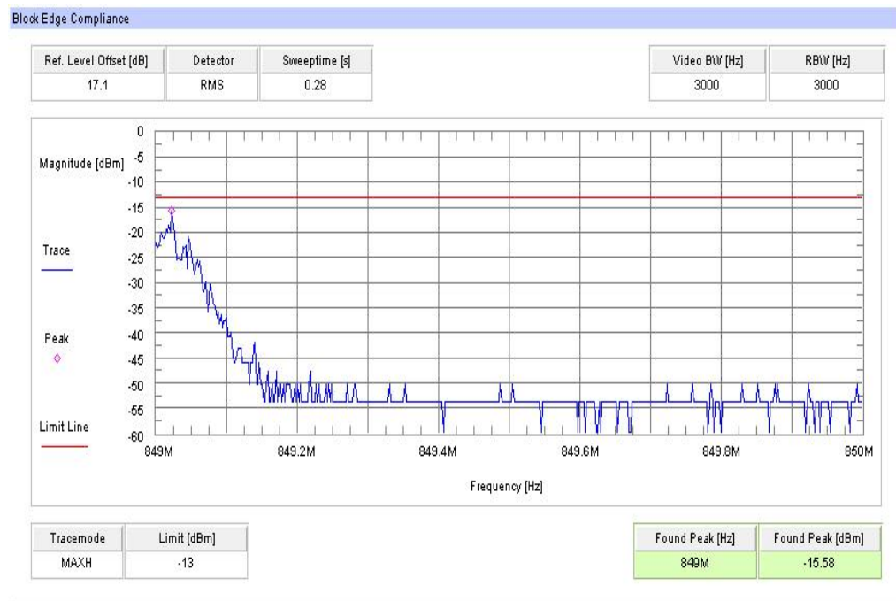
Plot 2: Channel 251 (GSM-mode)
