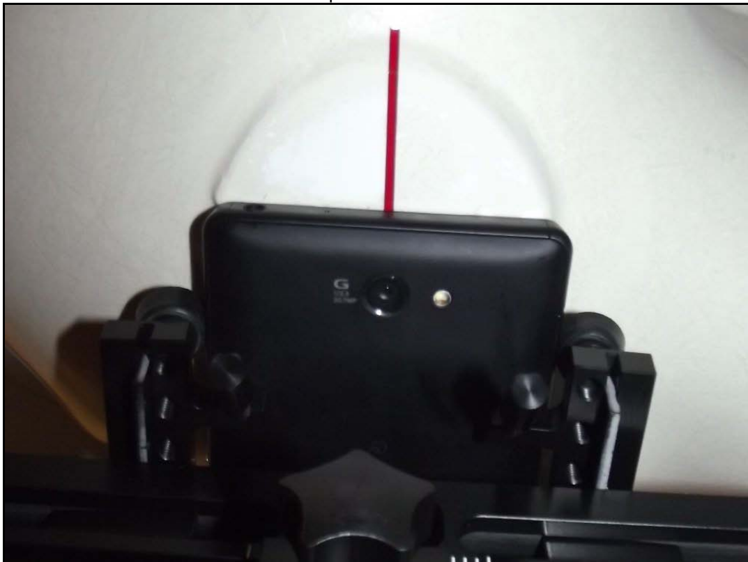
Photo 8: Test position left hand tilted 15°
