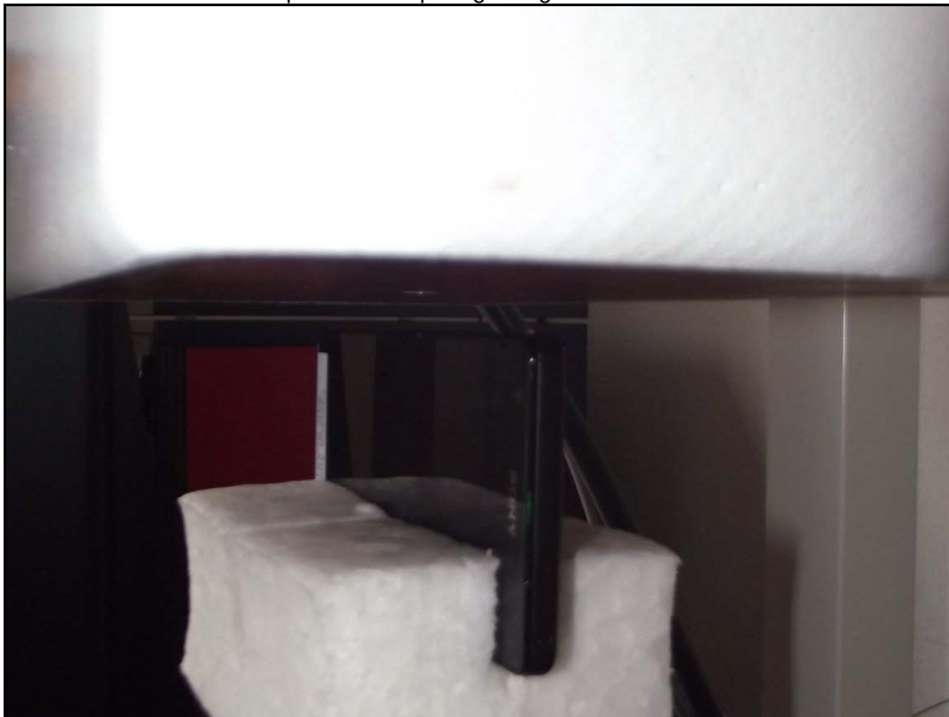
Photo 20: Test position hotspot left edge side with 10 mm distance
