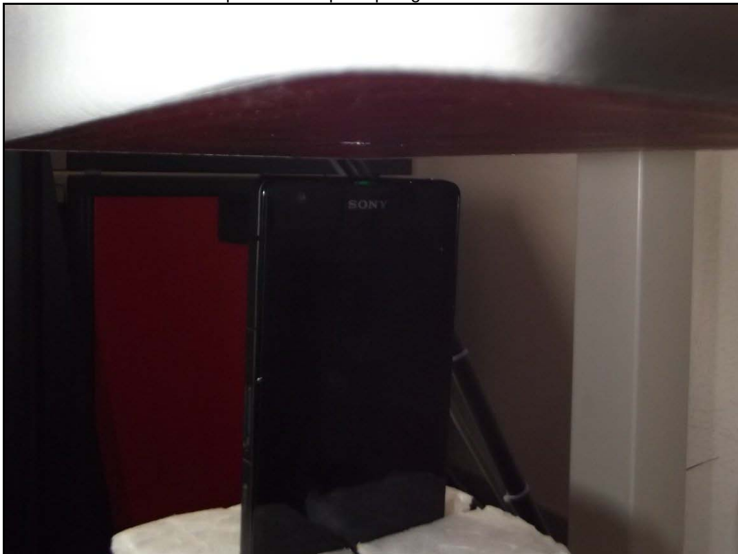
Photo 22: Test position hotspot bottom edge side with 10 mm distance
