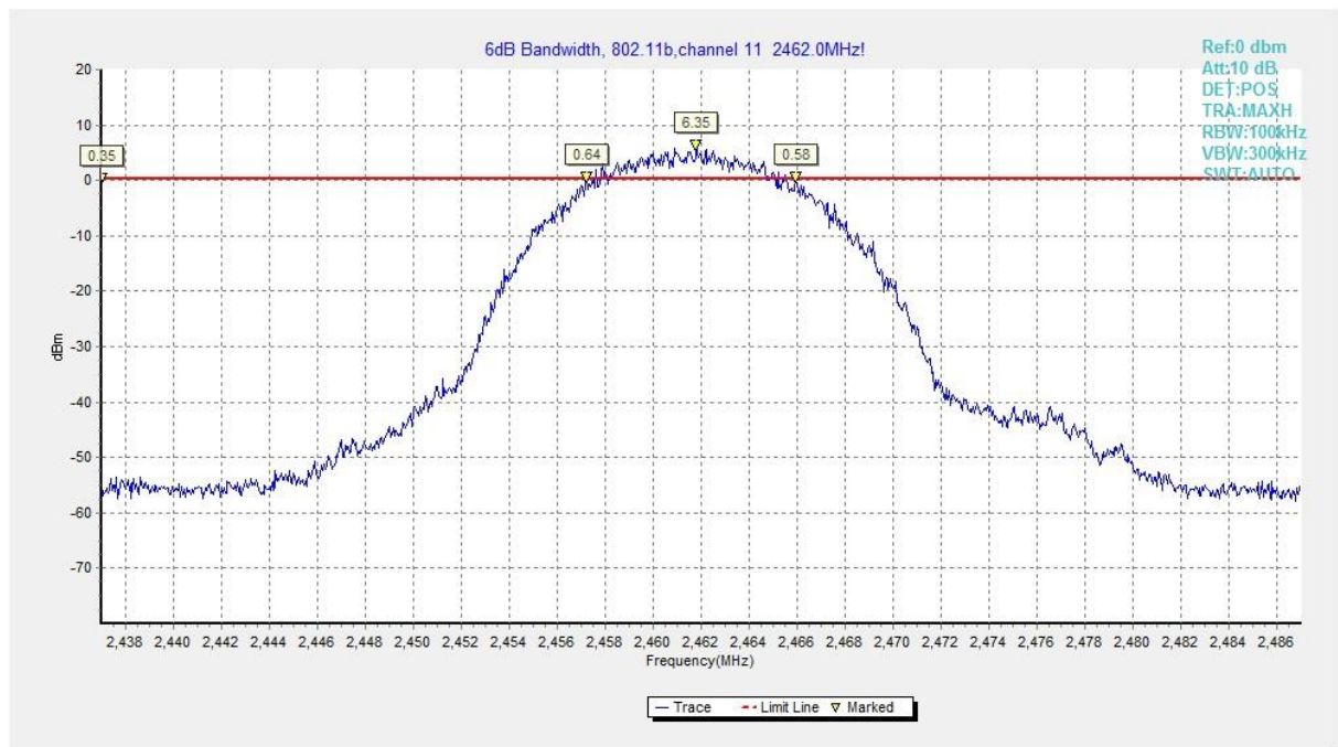
Fig.A.4.3 Occupied 6dB Bandwidth (802.11b, Ch 11)
