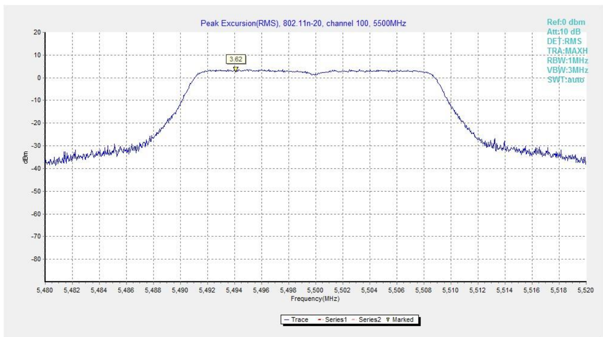
Fig. 193 Peak Excursions (802.11n-HT20, ch100, average)
