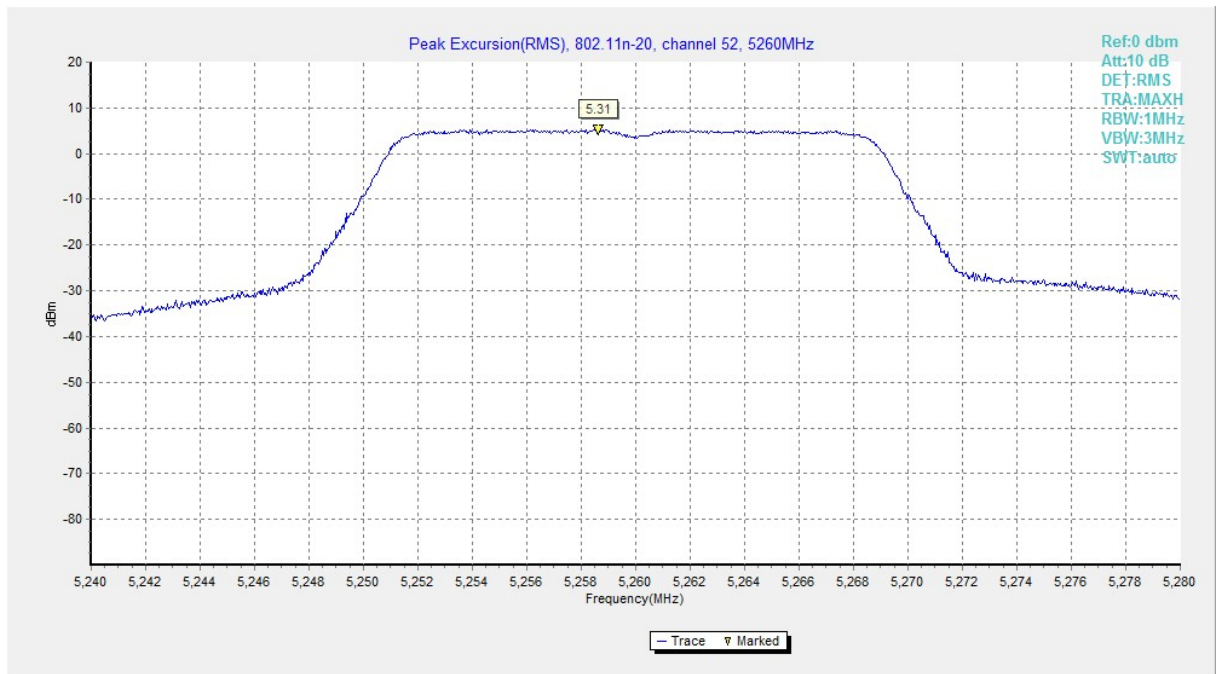
Fig. 167 Peak Excursions (802.11n-HT20, ch52, average)
