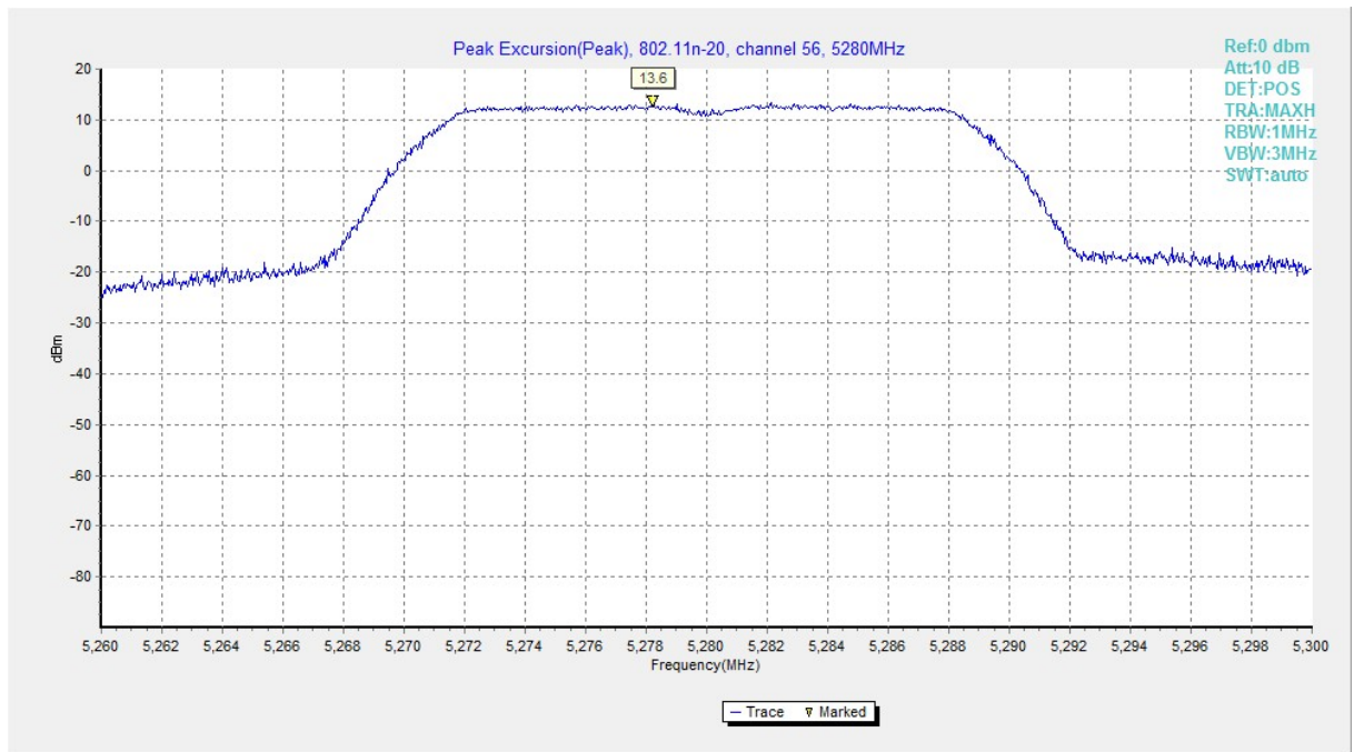
Fig. 165 Peak Excursions (802.11n-HT20, ch56, peak)
