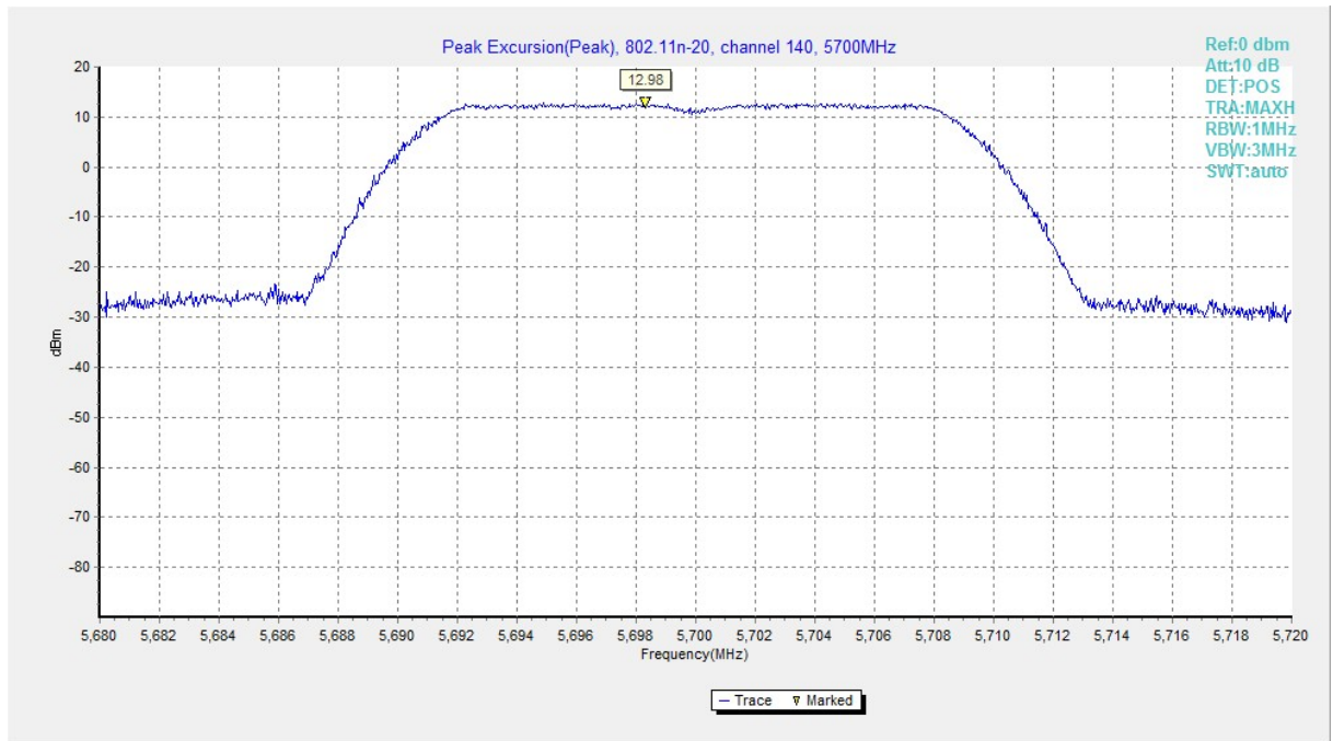
Fig. 172 Peak Excursions (802.11n-HT20, ch140, peak)
