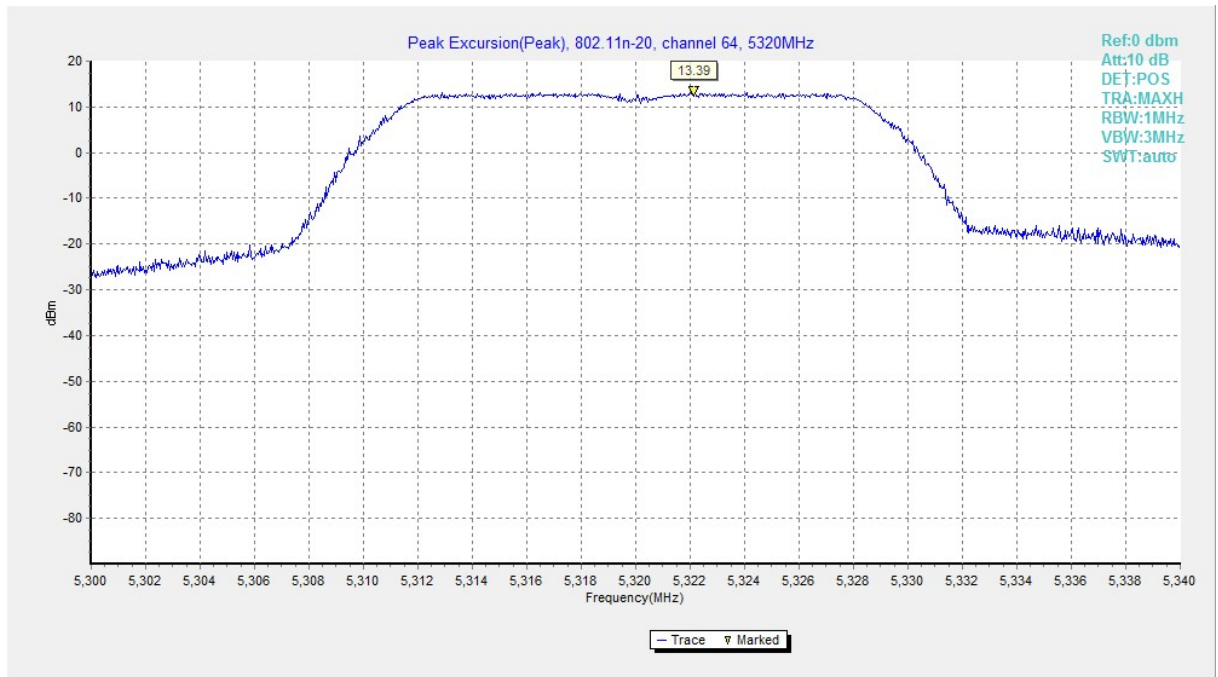
Fig. 166 Peak Excursions (802.11n-HT20, ch64, peak)
