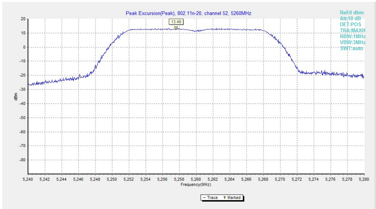
Fig. 164 Peak Excursions (802.11n-HT20, ch52, peak)
