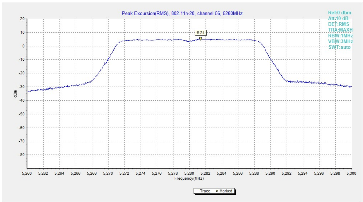
Fig. 168 Peak Excursions (802.11n-HT20, ch56, average)
