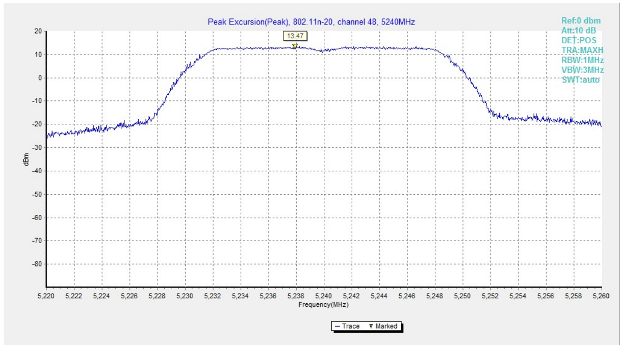
Fig. 160 Peak Excursions (802.11n-HT20, ch48, peak)
