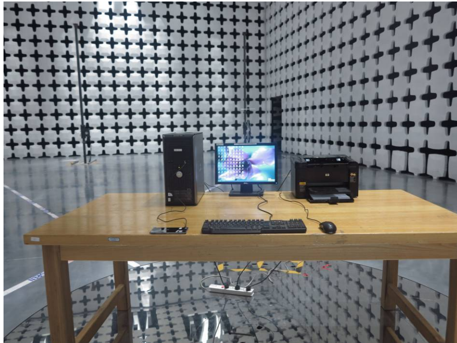
Pic.1 Radiated emission
