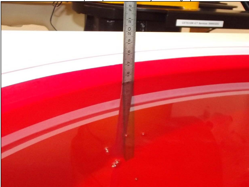
Photo 2: Liquid depth 850 MHz body simulating liquid
