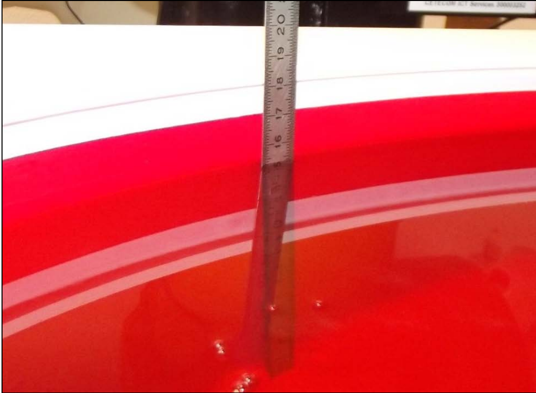
Photo 2: Liquid depth 850 MHz body simulating liquid
