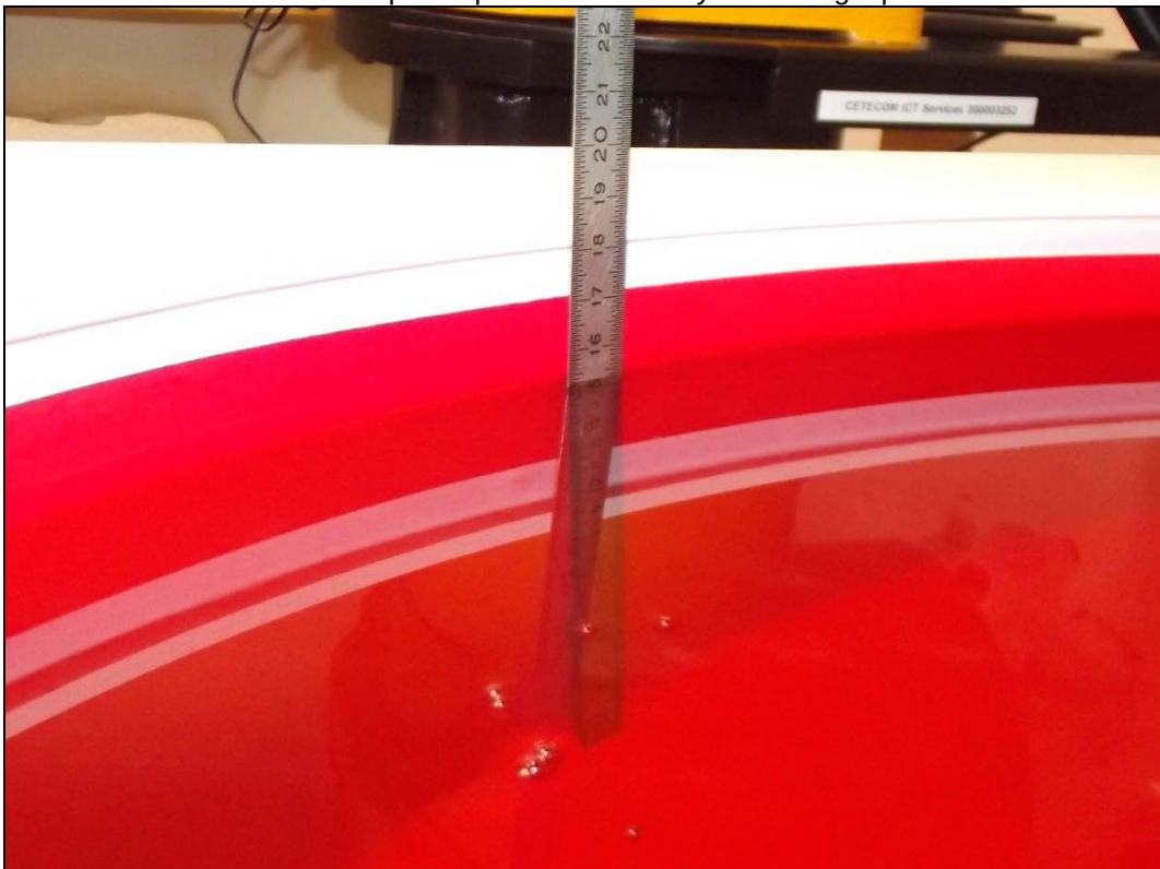
Photo 2: Liquid depth 850 MHz body simulating liquid
