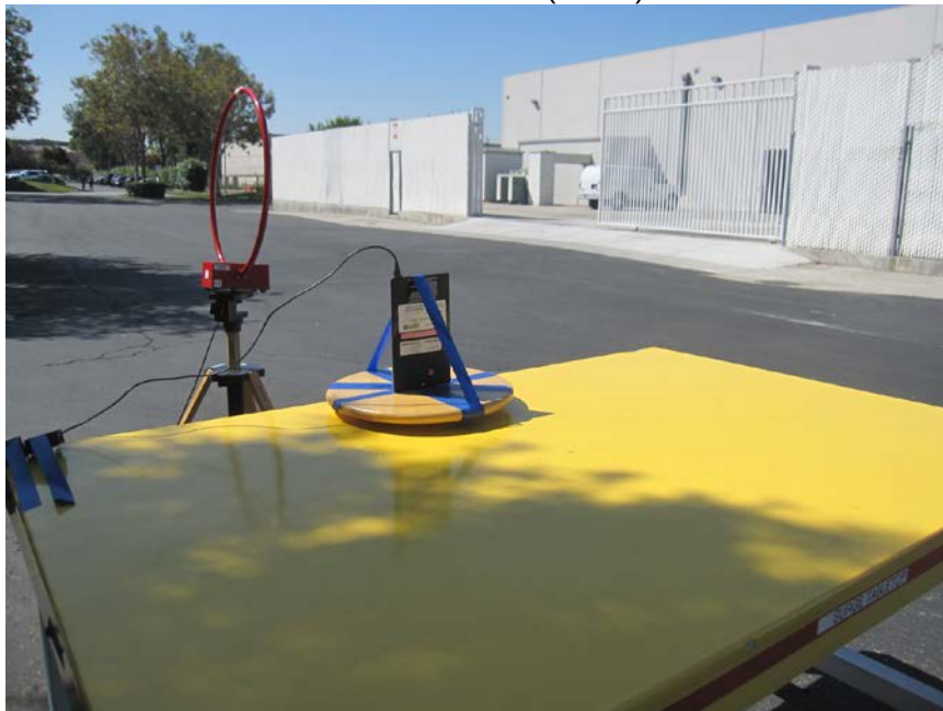
RADIATED EMISSIONS BELOW 30MHz (BACK)
