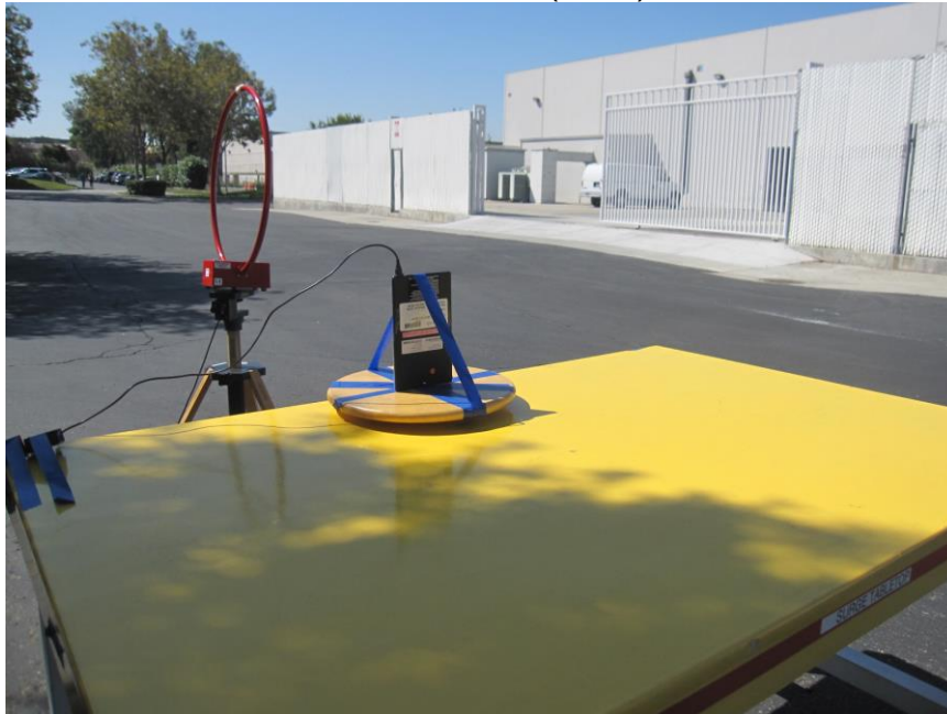
RADIATED EMISSIONS BELOW 30MHz (BACK)
