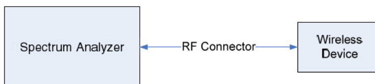
Figure 6-1. Test Instrument & Measurement Setup
