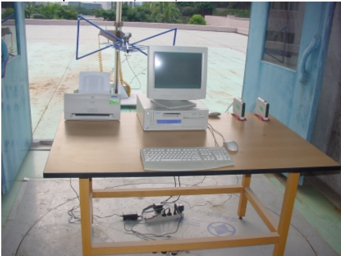
Photo 3 Test Setup for Radiated Test (Front View)
