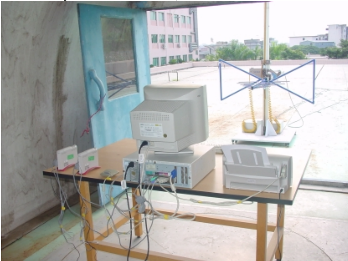
Photo 4 Test Setup for Radiated Test (Rear View)
