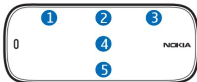
1. The signal strength of the cellular network at the current location, if this information is provided by the connected device; the higher the bar, the stronger the signal
